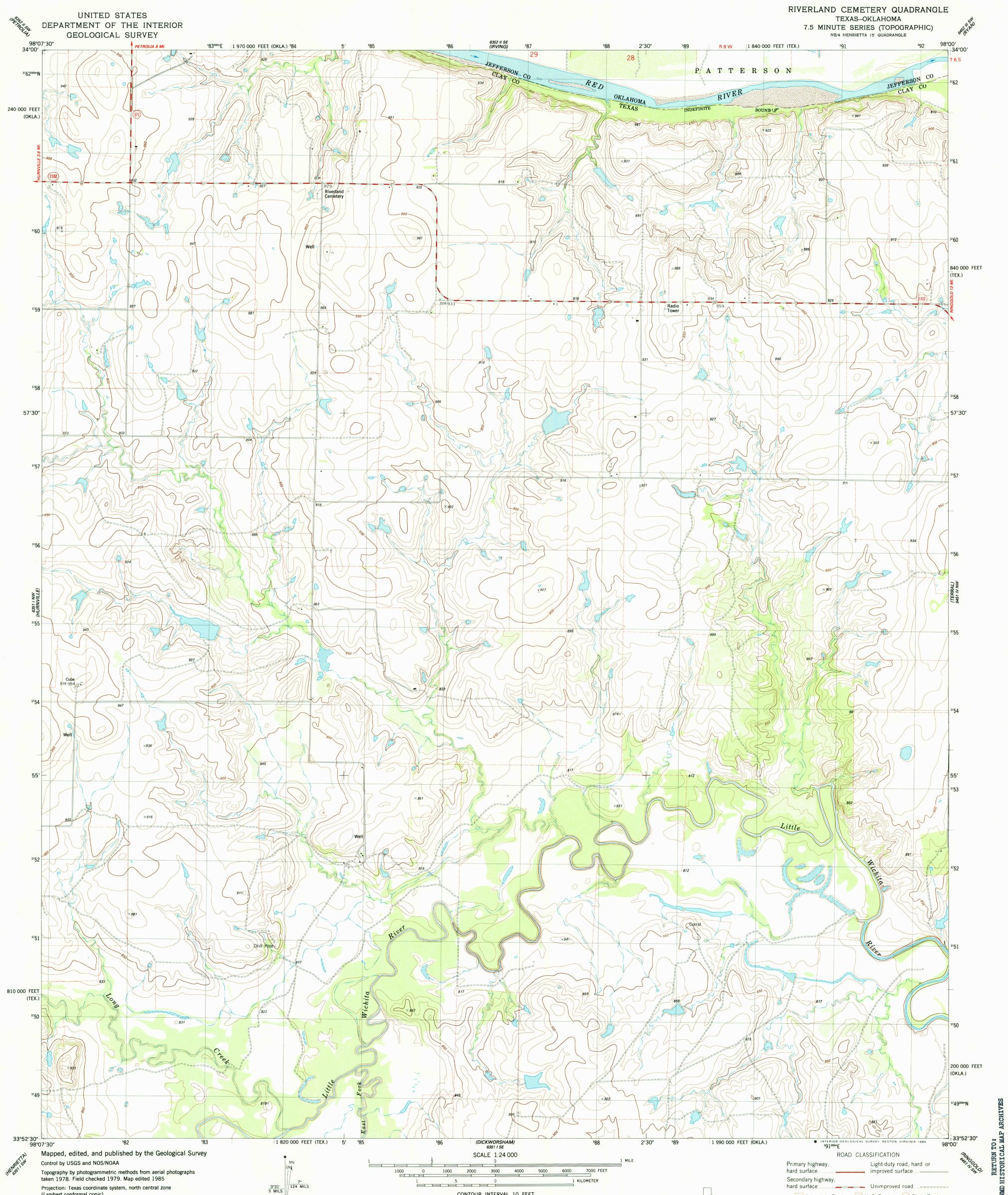
(Lambert conformal conic) 10,000-foot grid ticks based on Texas coordinate system, north central zone and Oklahoma coordinate system, south zone 1000-meter Universal Transverse Mercator grid, zone 14 1927 North American Datum To place on the predicted North American Datum 1983 move the projection lines 7 meters south and 30 meters east as shown by dashed corner tick.
