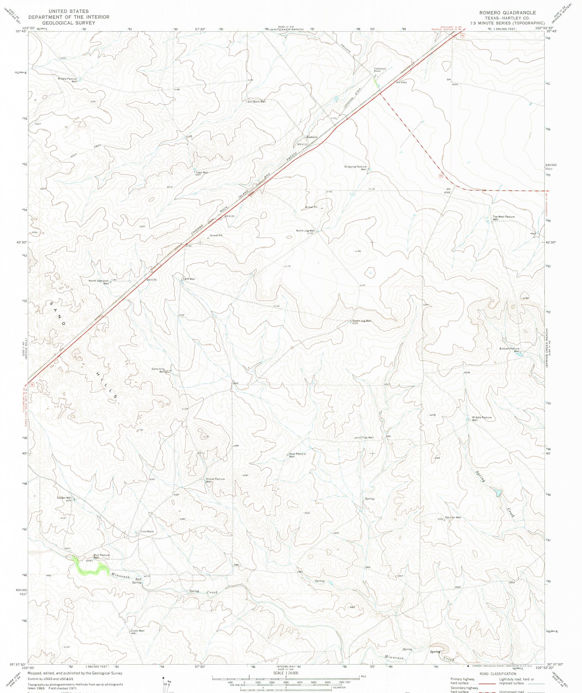
Polyconic projection. 1927 North American datum 10,000-foot grid based on Texas coordinate system, north zone 1000-meter Universal Transverse Mercator grid ticks, zone 13, shown in blue
