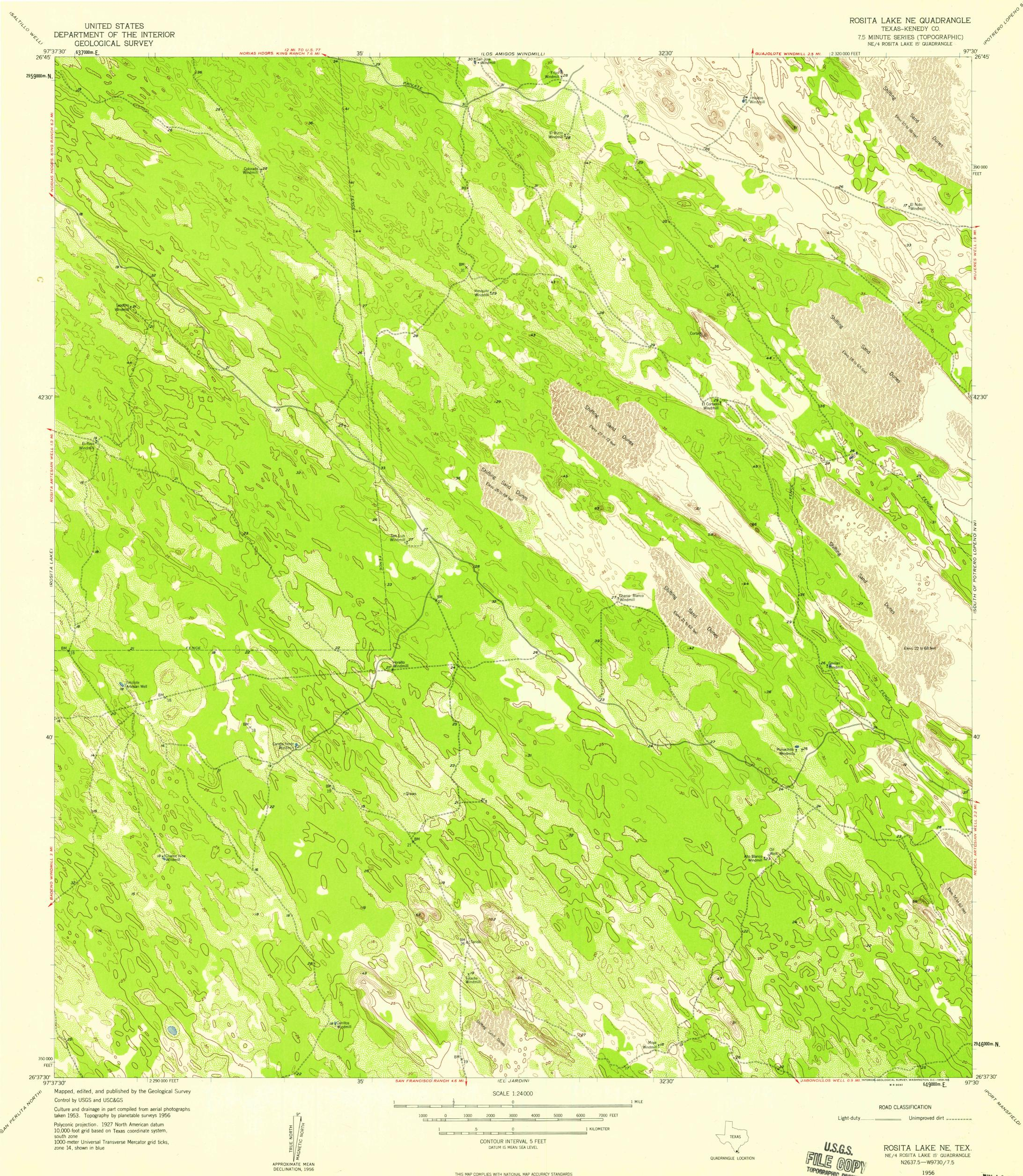
Polyconic projection. 1927 North American datum 10,000-foot grid based on Texas coordinate system, south zone 1000-meter Universal Transverse Mercator grid ticks, zone 14, shown in blue
