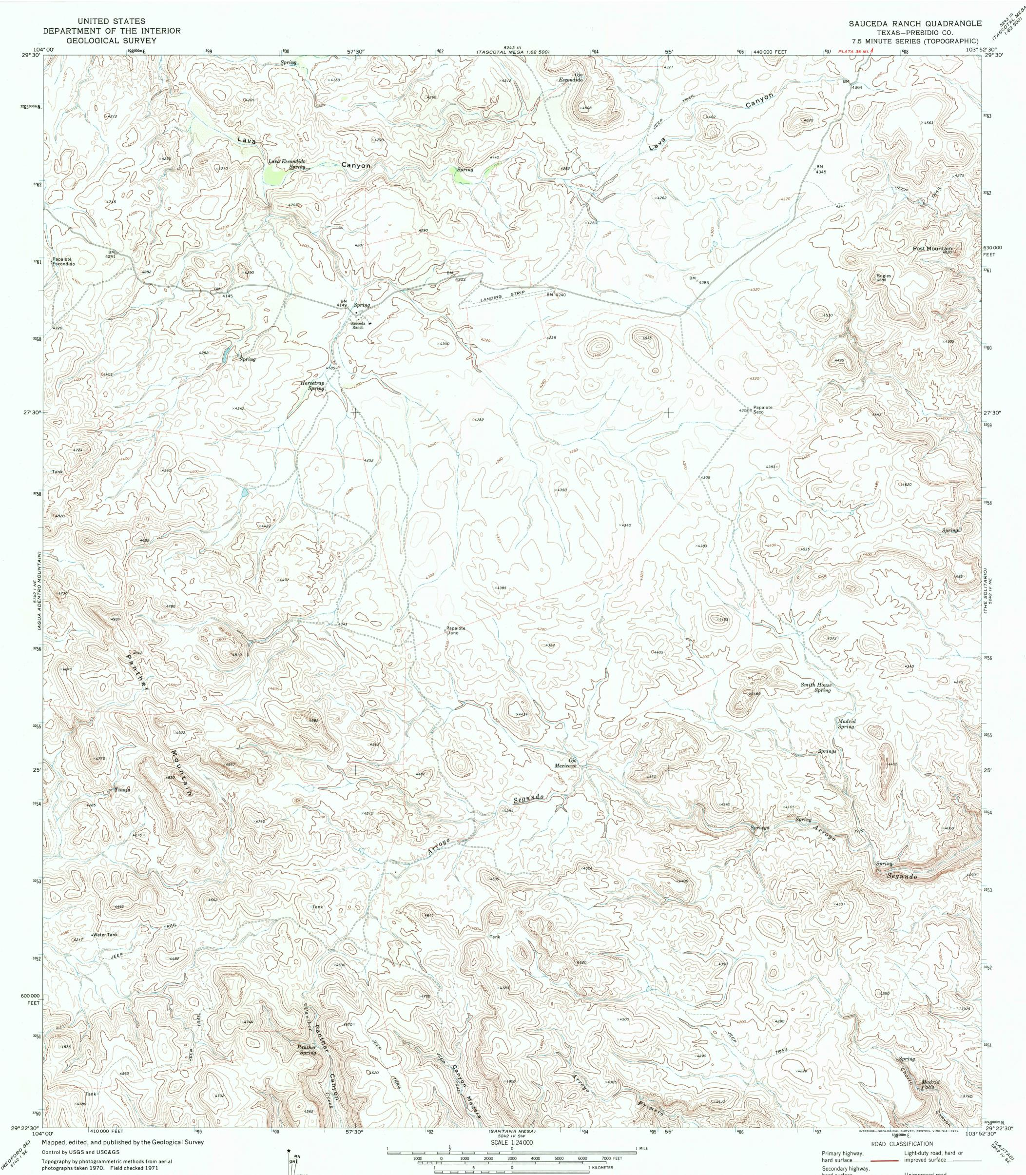
Projection and 10,000-foot grid ticks: Texas coordinate system, south central zone (Lambert conformal conic) 1000-meter Universal Transverse Mercator grid ticks, zone 13, shown in blue. 1927 North American datum
