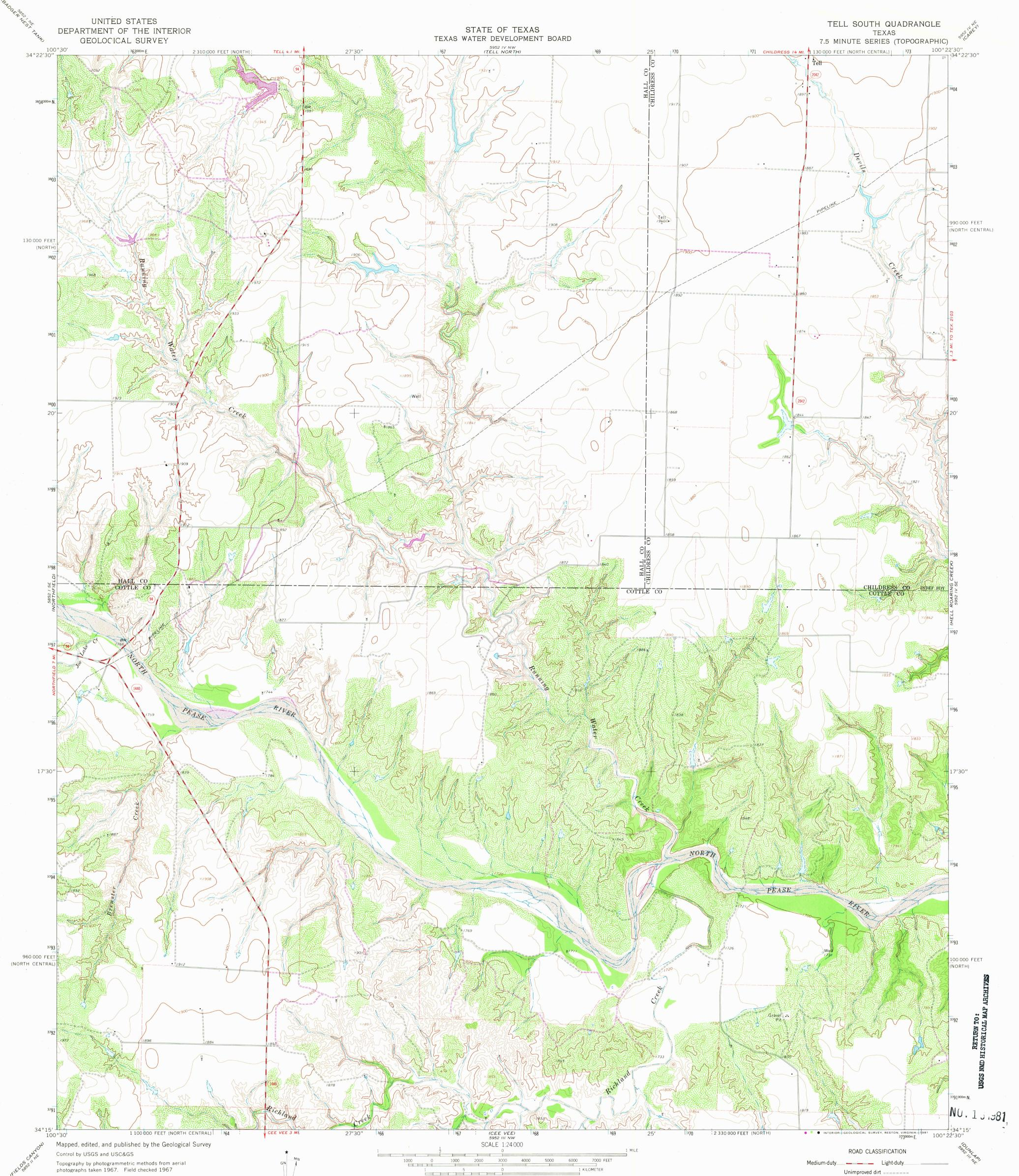
Polyconic projection. 1927 North American datum 10,000-foot grids based on Texas coordinate system, north central and north zones 1000-meter Universal Transverse Mercator grid ticks, zone 14, shown in blue Fine red dashed lines indicate selected fence lines To place on the predicted North American Datum 1983 move the projection lines 3 meters south and 37 meters east as shown by dashed corrier ticks
