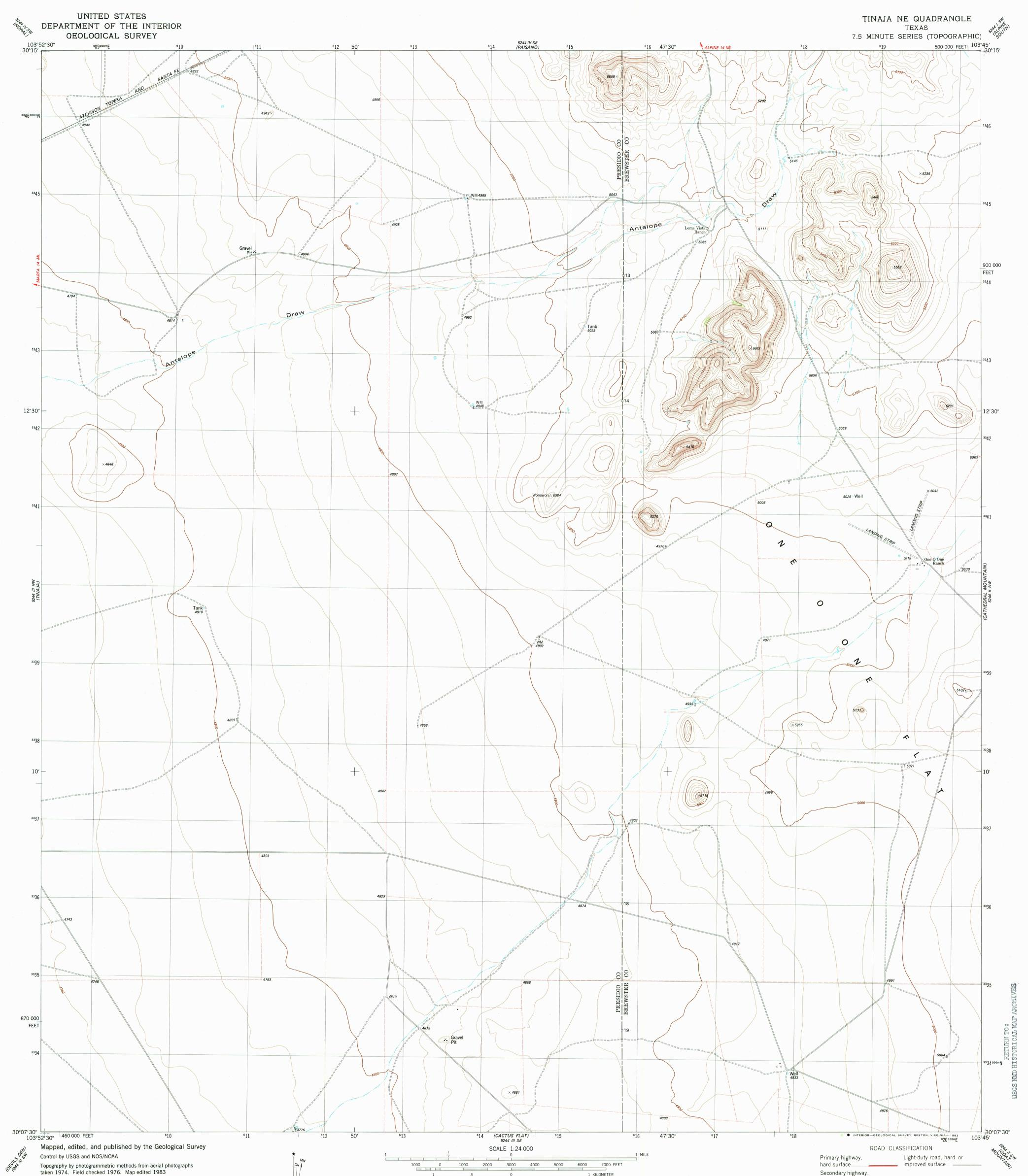
Projection and 10,000-foot grid ticks: Texas coordinate system, south central zone (Lambert conformal conic) 1000-meter Universal Transverse Mercator grid, zone 13 1927 North American datum To place on the predicted North American Datum 1983 move the projection lines 15 meters south and 44 meters east as shown by dashed corner ticks Fine red dashed lines indicate selected fence lines
