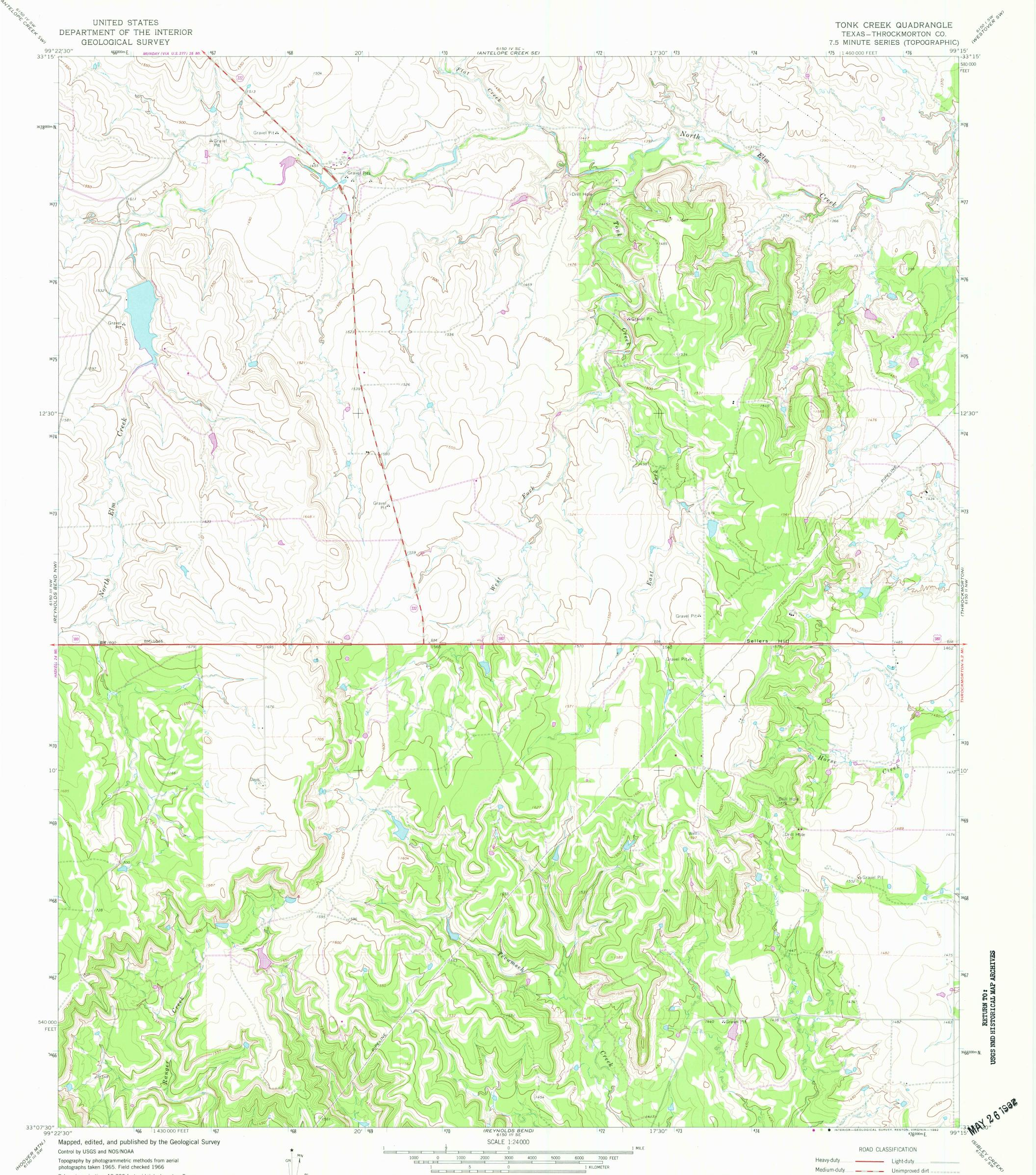
Polyconic projection. 10,000-foot grid ticks based on Texas coordinate system, north central zone. 1000-meter Universal Transverse Mercator grid ticks, zone 14, shown in blue 1927 North American Datum. To place on the predicated North American Datum 1983 move the projection lines 8 meters south and 33 meters east as shown by dashed corner ticks
