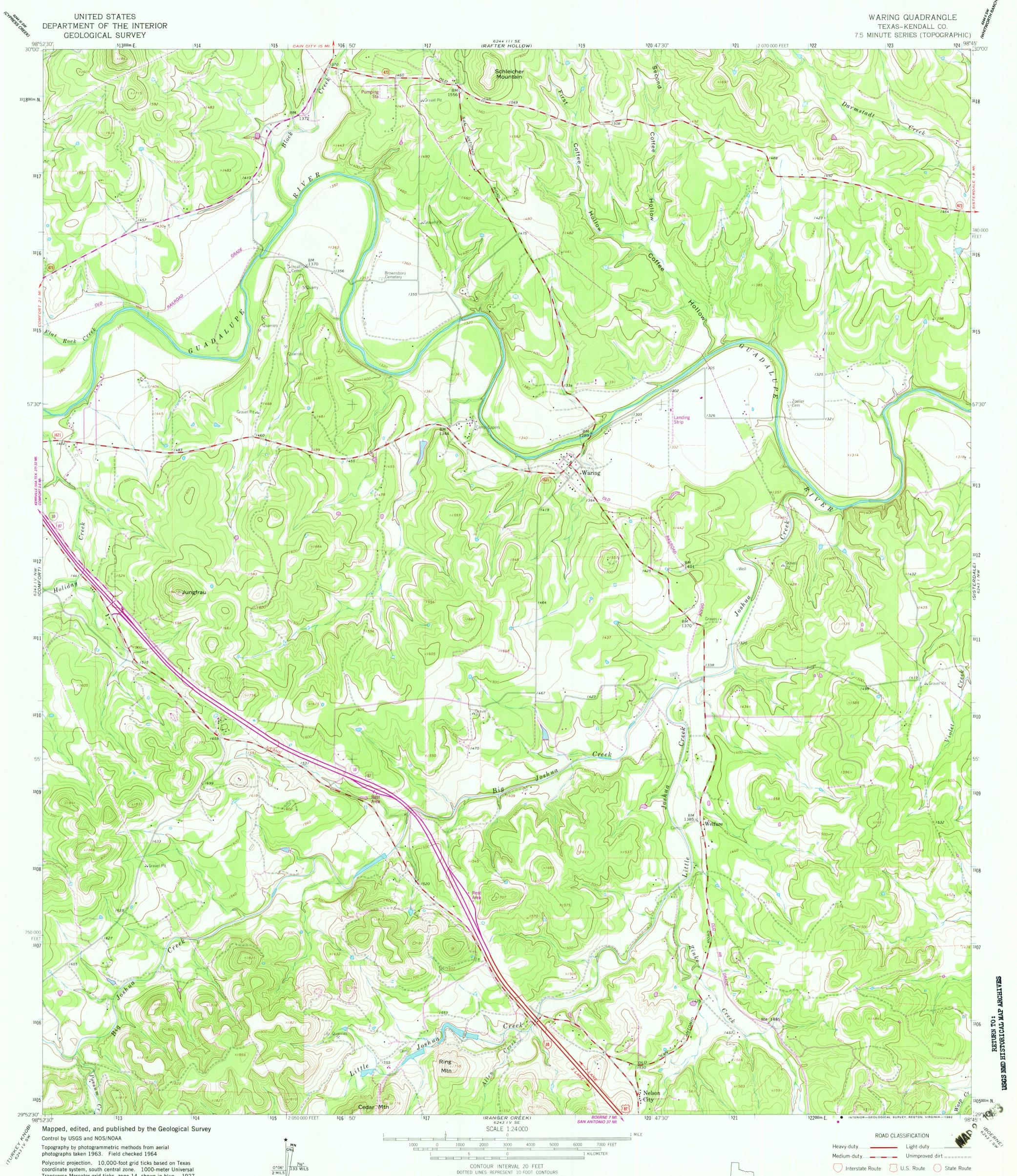
coordinate system, south central zone. 1000-meter Universal Transverse Mercator grid ticks, zone 14, shown in blue. 1927 North American Datum. To place on the predicted North American Datum 1983 move the projection lines 19 meters south and 30 meters east as shown by da hed corner ticks
