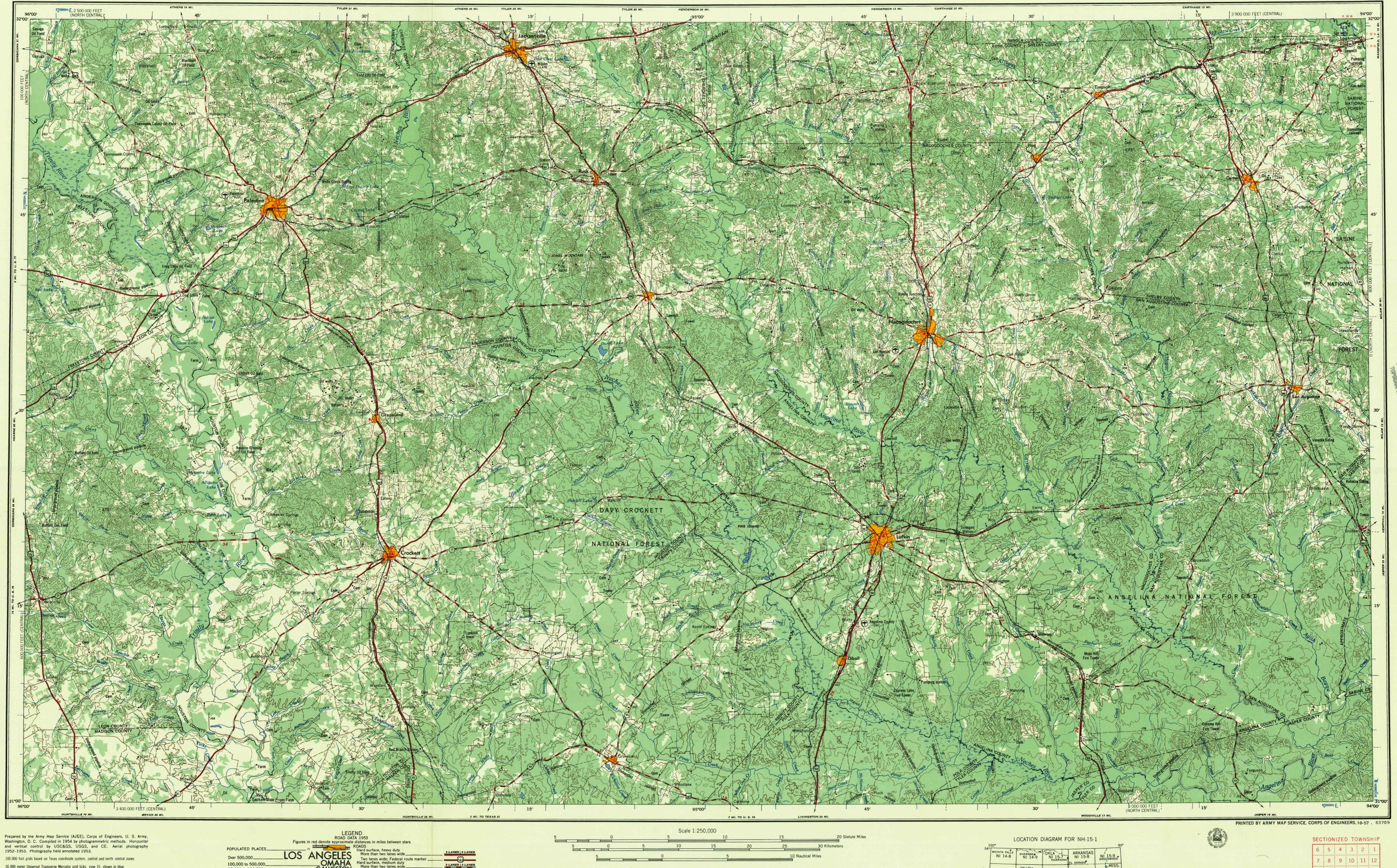
Prepared by the Army Map Service (AJEE), Corps of Engineers, U. S. Army, Washington, D. C. Compiled in 1954 by photogrammetric methods. Horizontal and vertical control by USC&GS, USGS, and CE. Aerial photography 1952–1953. Photography field annotated 1953.
