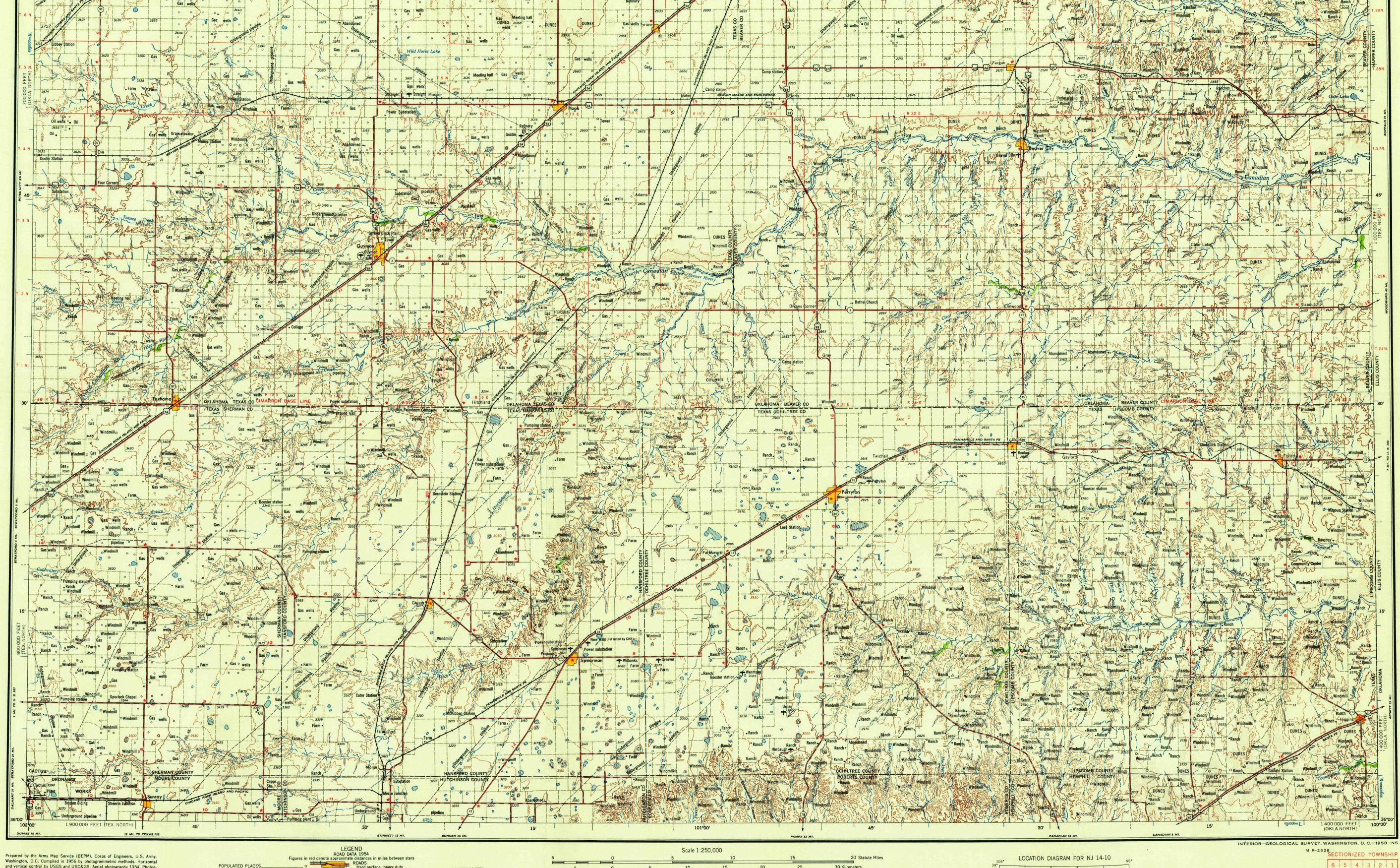
Prepared by the Army Map Service (BEPM), Corps of Engineers, U.S. Army, Washington, D.C. Compiled in 1956 by photogrammetric methods. Horizontal and vertical control by USGS and USC&GS. Aerial photography 1954. Photogram raphy field annotated 1954.  $100,\!000\!\operatorname{-foot}$  grids based on Texas coordinate system, north zone and Oklahoma coordinate system, north zone 10,000-meter Universal Transverse Mercator grid ticks, zone 14, shown in blue
