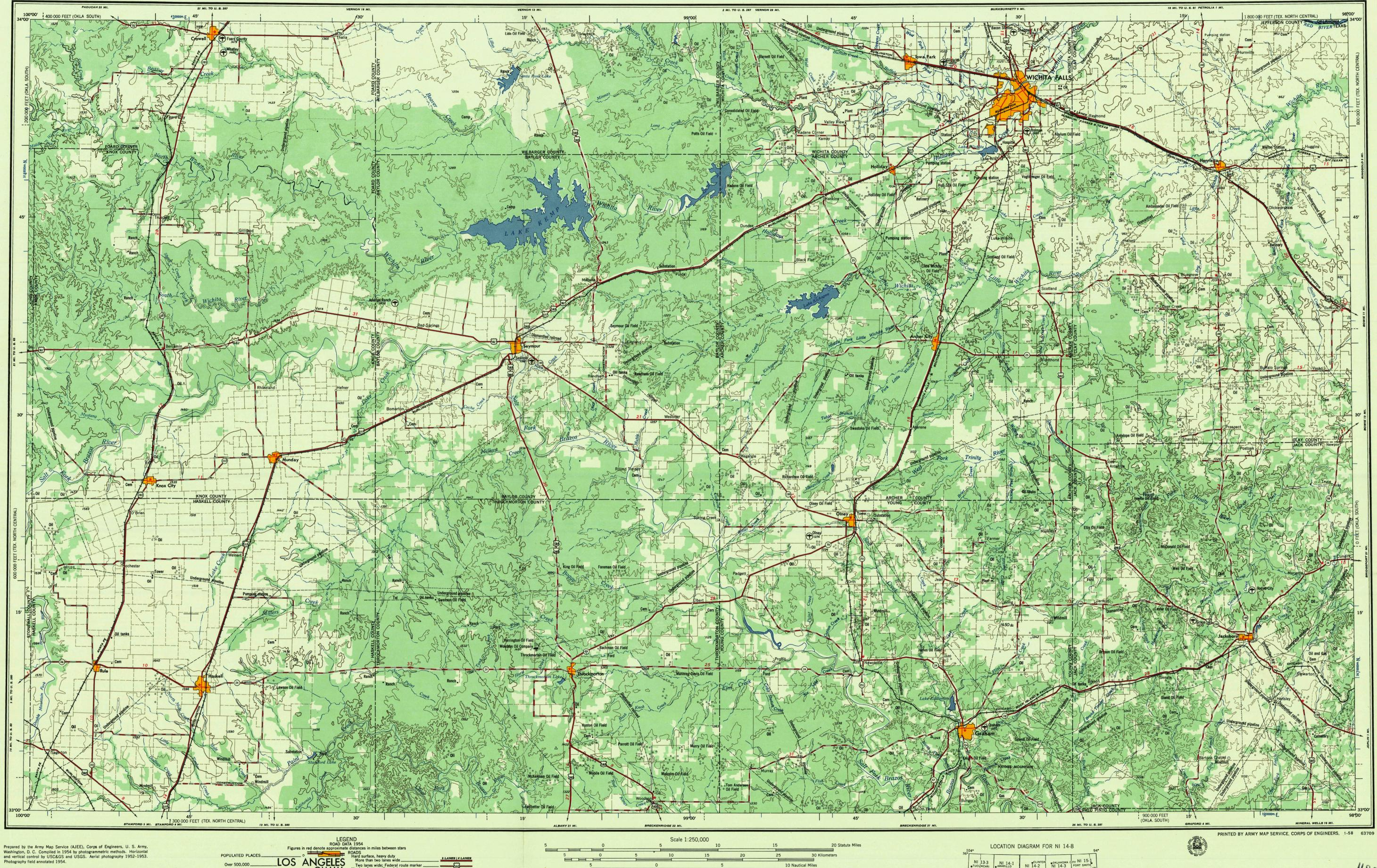
100,000 foot grids based on Texas coordinate system, north central zone and Oklahoma coordinate system, south zone 10,000 meter Universal Transverse Mercator grid ticks, zone 14, shown in blue
