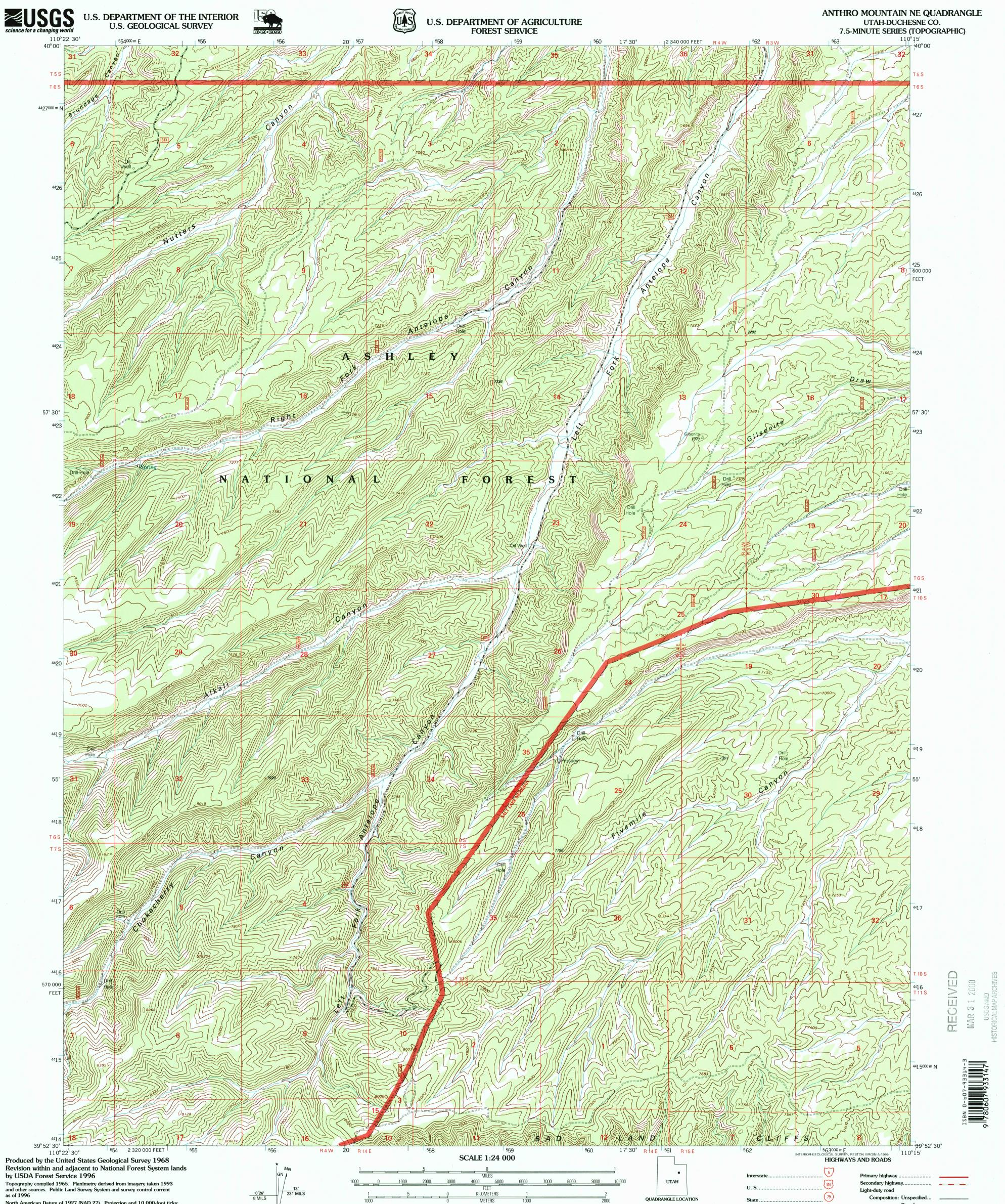
North American Datum of 1927 (NAD 27). Projection and 10 000-foot ticks Utah coordinate system, central zone (Lambert conformal conic) Blue 1000-meter Universal Transverse Mercator ticks, zone 12
