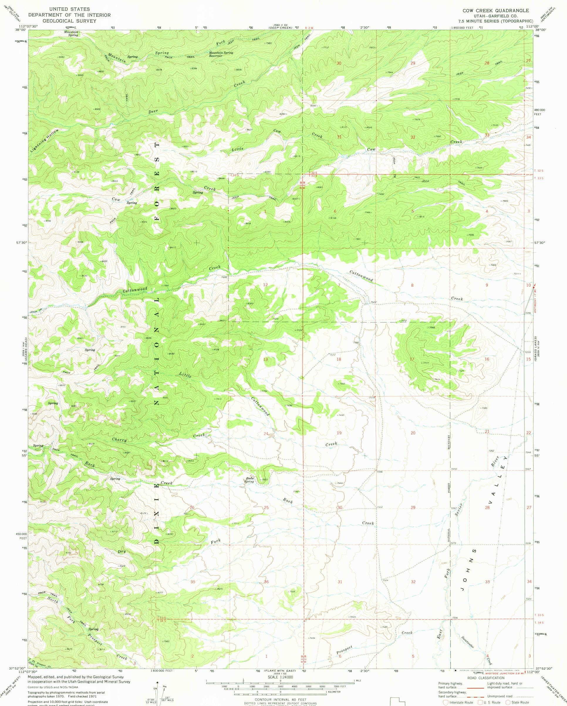
system, south zone (Lambert conformal conic) 1000-meter Universal Transverse Mercator grid ticks, zone 12, shown in blue. 1927 North American datum Fine red dashed lines indicate selected fence lines
