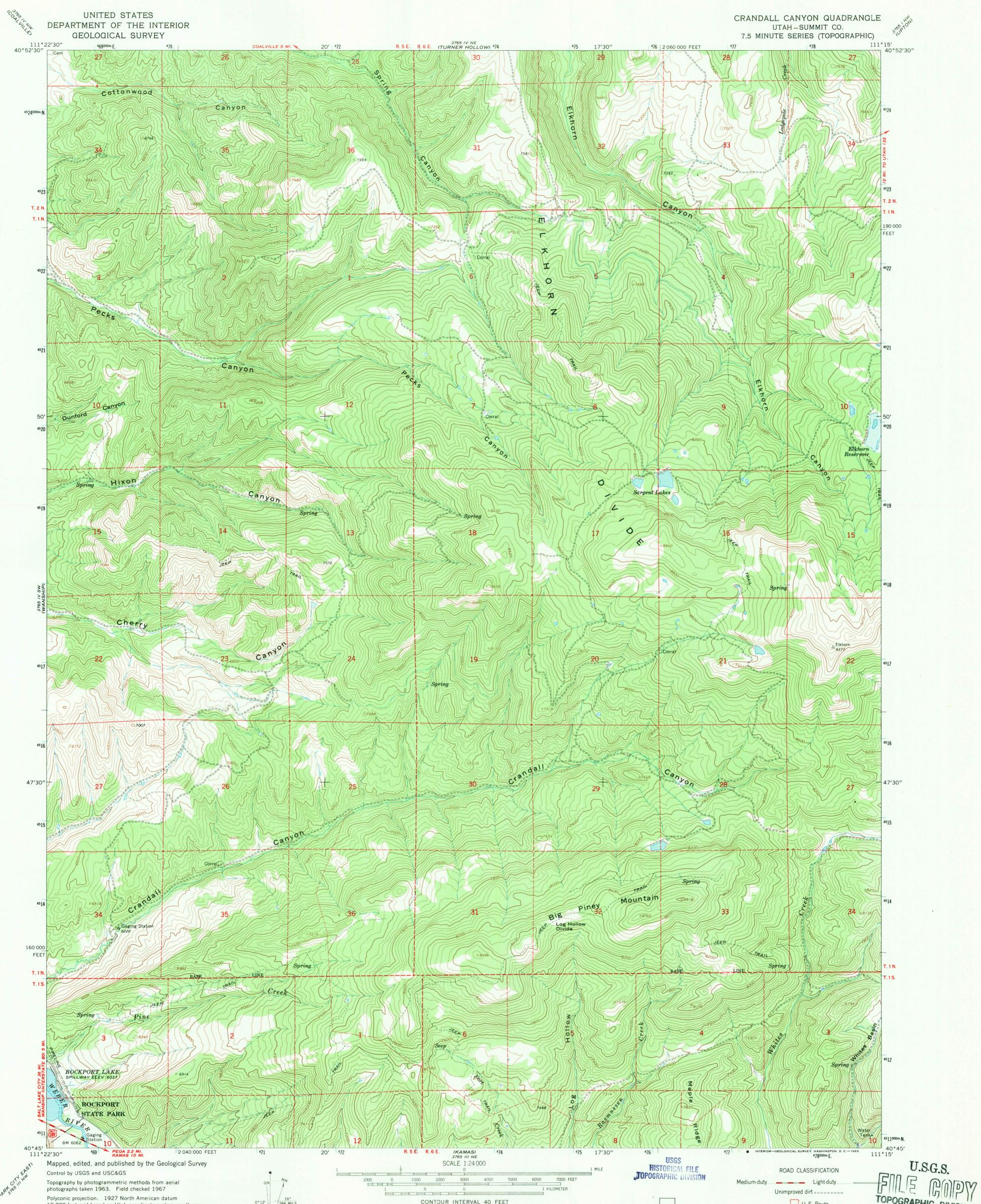
Polyconic projection. 1927 North American datum 10,000-foot grid based on Utah coordinate system, north zone 1000-meter Universal Transverse Mercator grid ticks, zone 12, shown in blue
