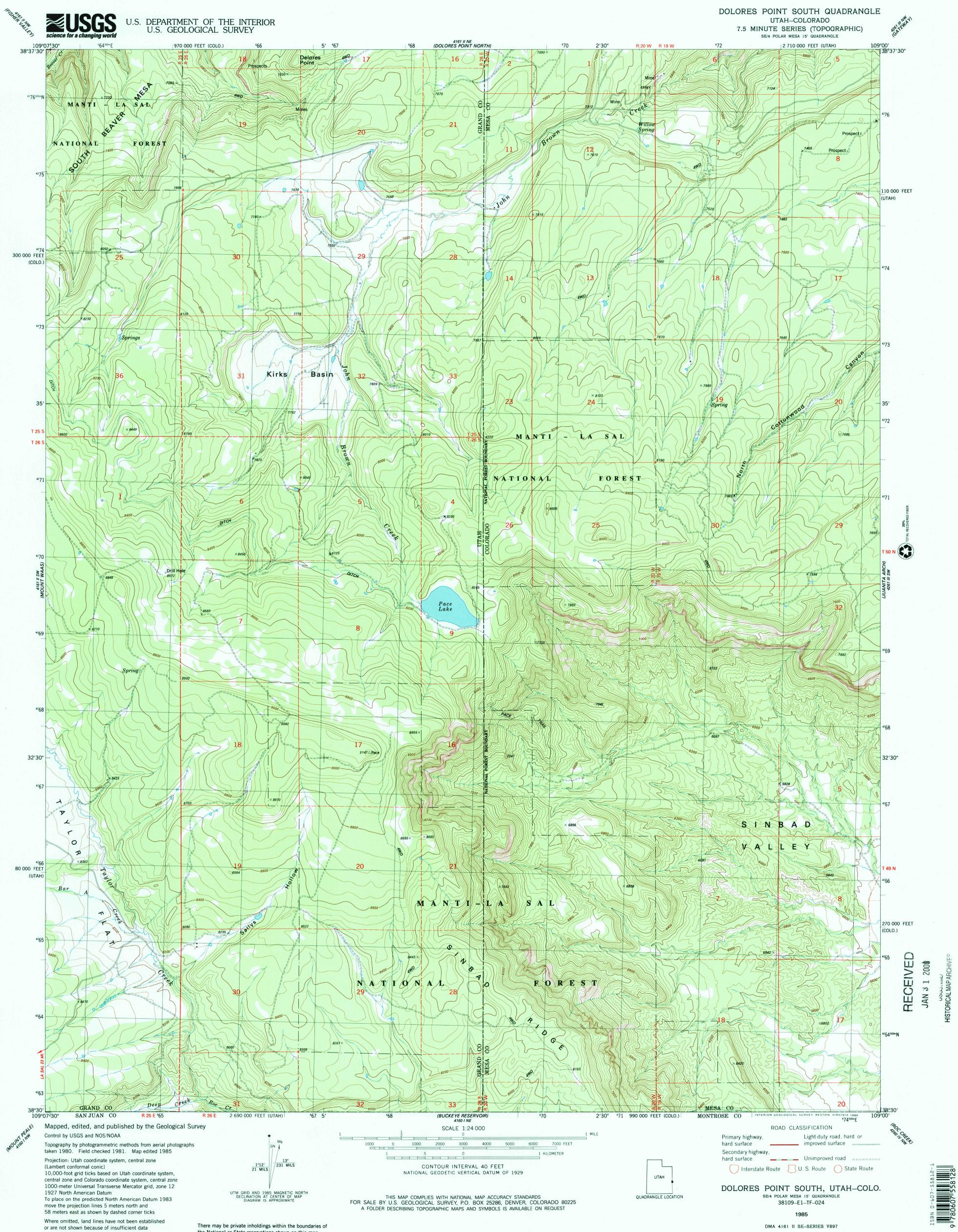
10,000-foot grid ticks based on Utah coordinate system, central zone and Colorado coordinate system, central zone 1000-meter Universal Transverse Mercator grid, zone 12 1927 North American Datum To place on the predicted North American Datum 1983 move the projection lines 5 meters north and 58 meters east as shown by dashed corner ticks
