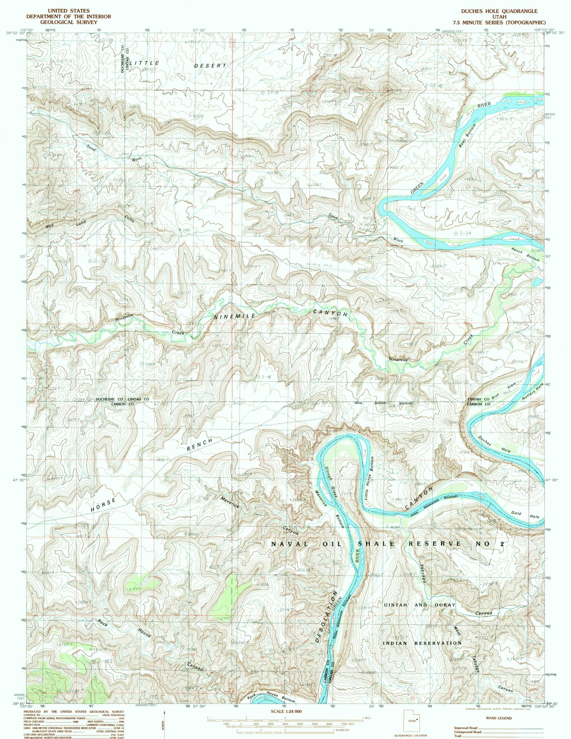
VERTICAL DATUM NATIONAL GEODETIC VERTICAL DATUM OF 1929 HORIZONTAL DATUM NATIONAL GEODETIC VERTICAL DATUM OF 1929 HORIZONTAL DATUM 1927 NORTH AMERICAN DATUM To place on the predicted North American Datum of 1983, move the projection lines as shown by dashed corner ticks (7 meters north and 60 meters east) There may be private inholdings within the boundaries of any Federal and State Reservations shown on this map Where omitted, land lines have not been established field
