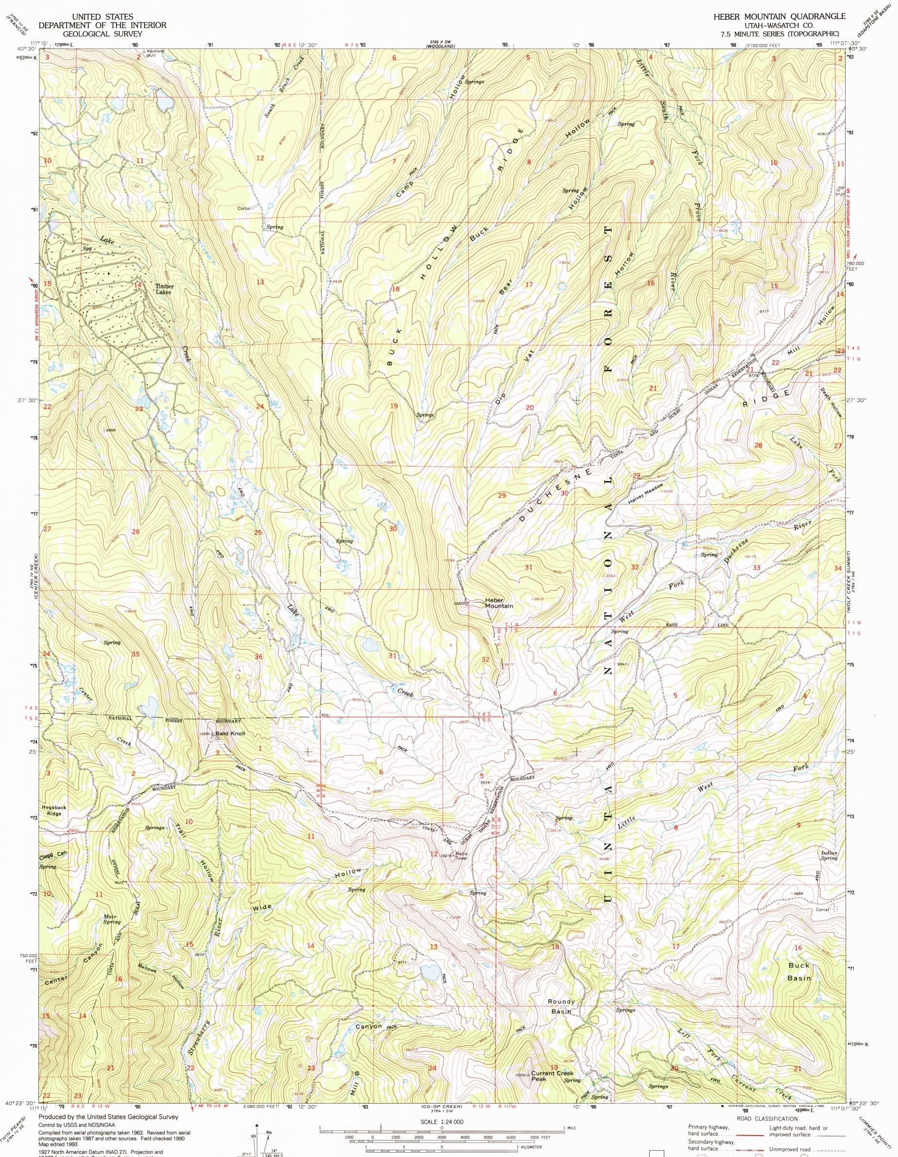
10000-foot ticks: Utah Coordinate System, central zone (Lambert Conformal Conic) Blue 1000-meter Universal Transverse Mercator ticks, zone 12 North American Datum of 1983 (NAD 83) is shown by dashed corner ticks. The values of the shift between NAD 27 and NAD 83 for 7.5-minute intersections are given in USGS Bulletin 1875 UTM GRID AND 1993 MAGNETIC NORTH DECLINATION AT CENTER OF SHEET There may be private inholdings within the boundaries of the
