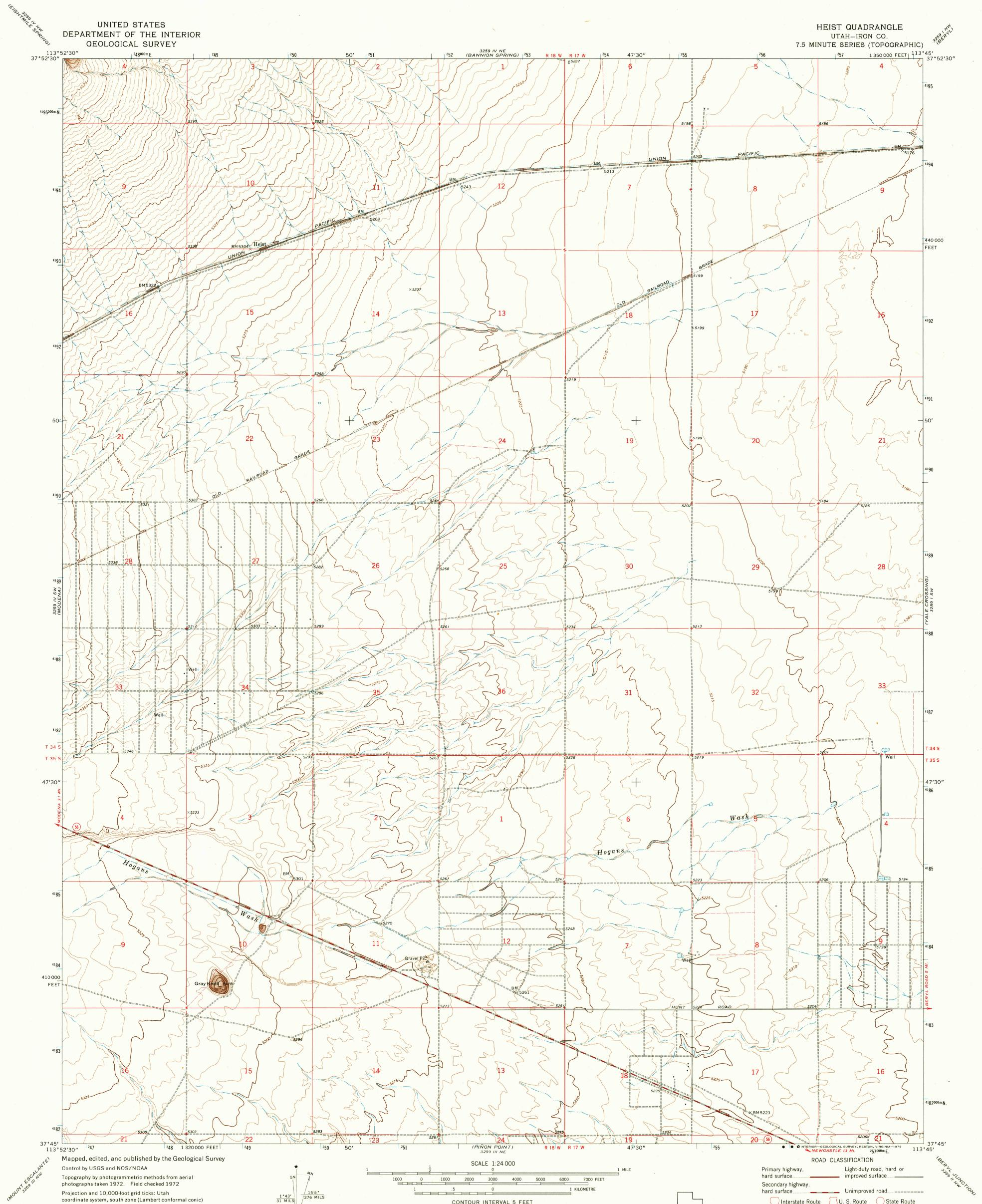
coordinate system, south zone (Lambert conformal conic) 1000-metre Universal Transverse Mercator grid ticks, zone 12, shown in blue. 1927 North American datum
