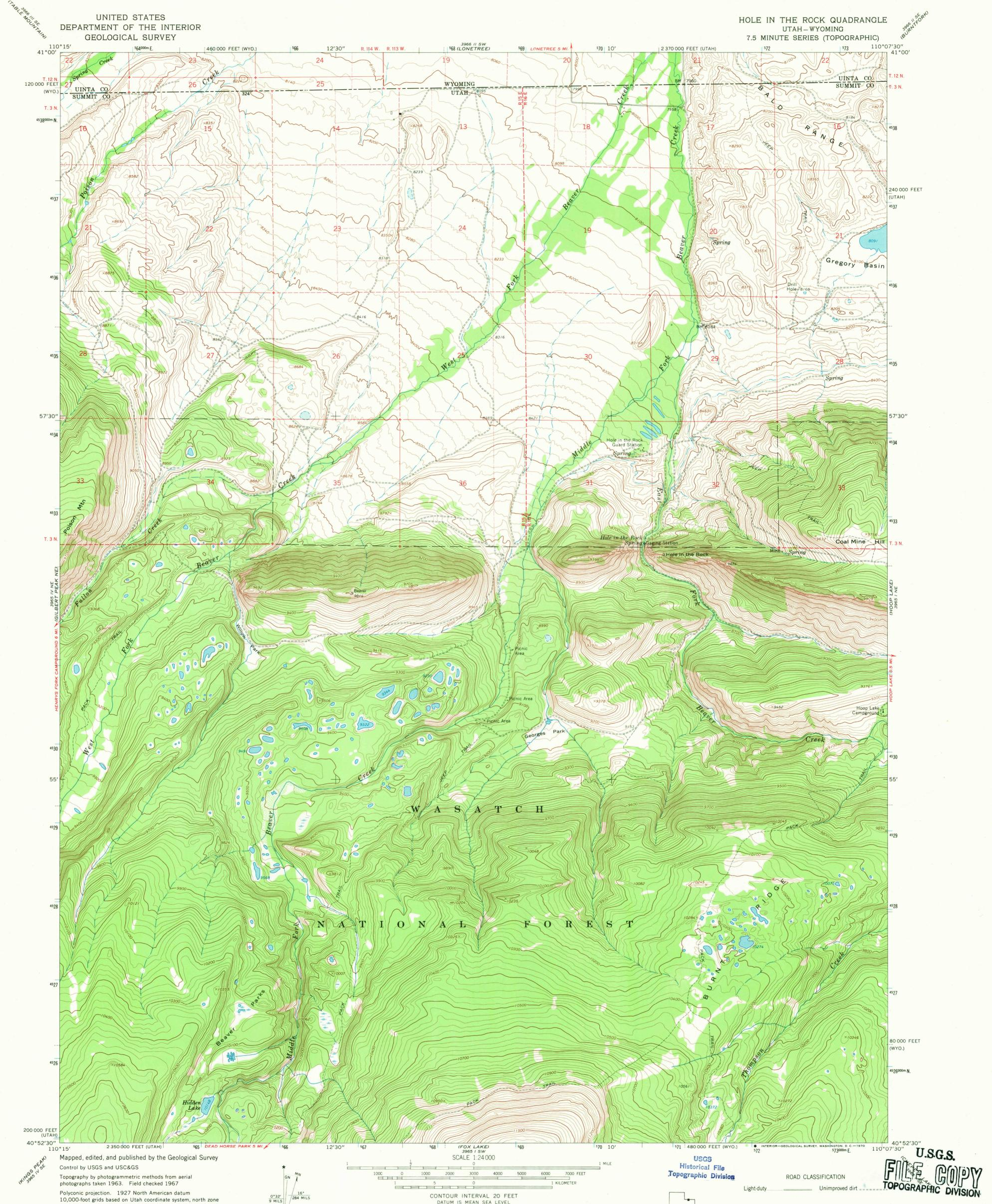
10,000-foot grids based on Utah coordinate system, north zone and Wyoming coordinate system, west zone 1000-meter Universal Transverse Mercator grid ticks, zone 12, shown in blue
