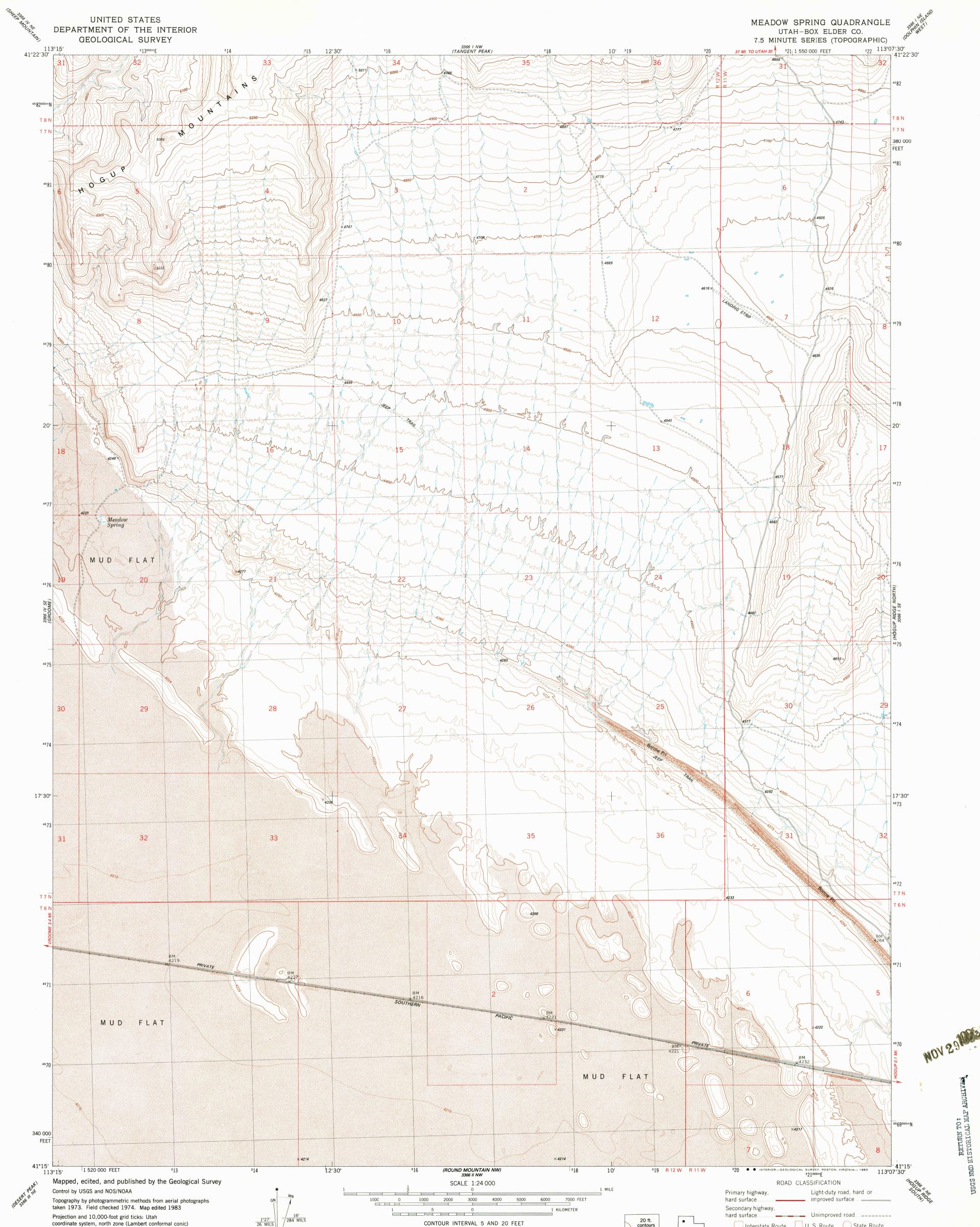
coordinate system, north zone (Lambert conformal conic) 1000-meter Universal Transverse Mercator grid, zone 12 1927 North American datum To place on the predicted North American Datum 1983 move the projection lines 11 meters north and 69 meters east as shown by dashed corner ticks
