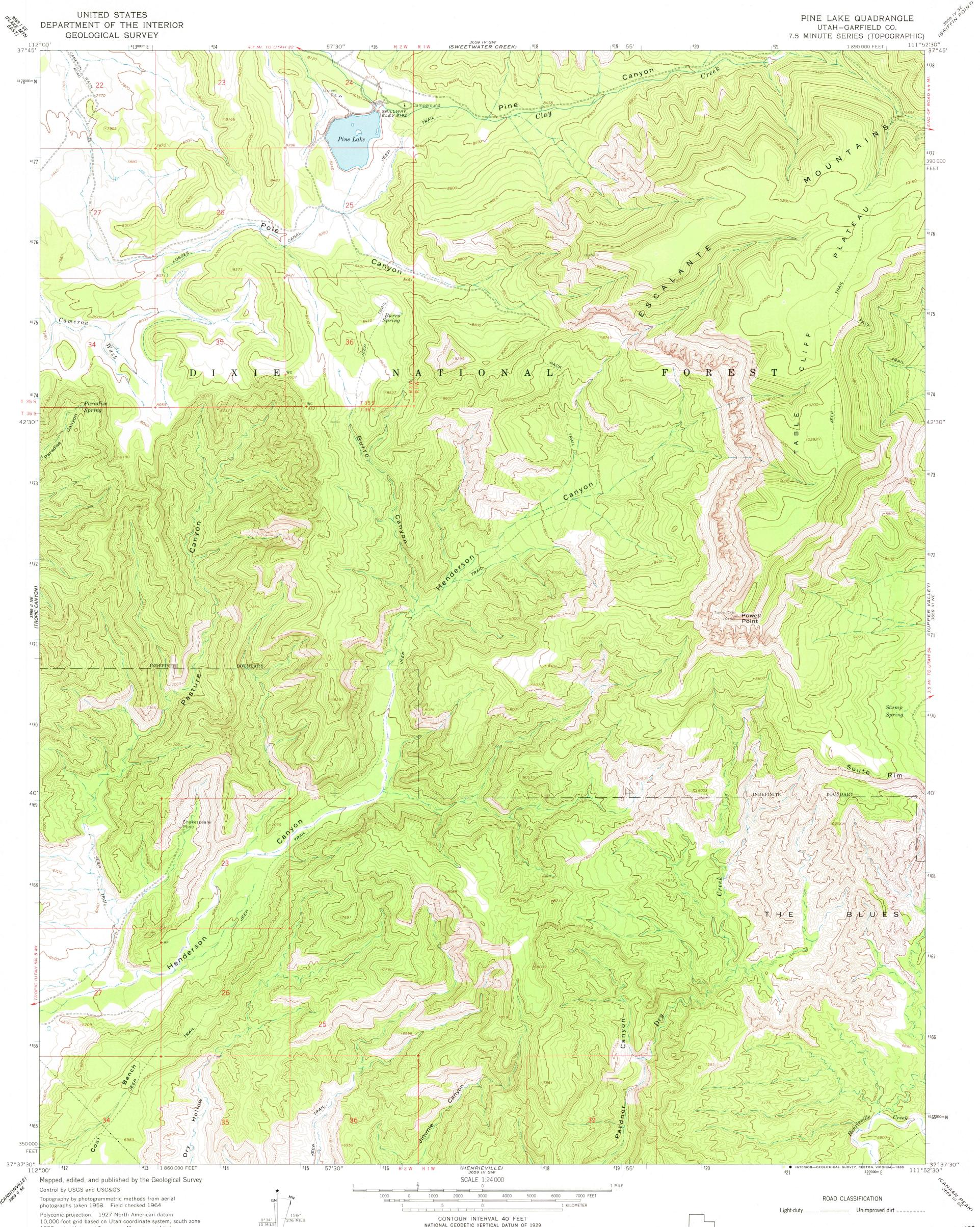
10,000-foot grid based on Utah coordinate system, south zone 1000-meter Universal Transverse Mercator grid ticks, zone 12, shown in blue
