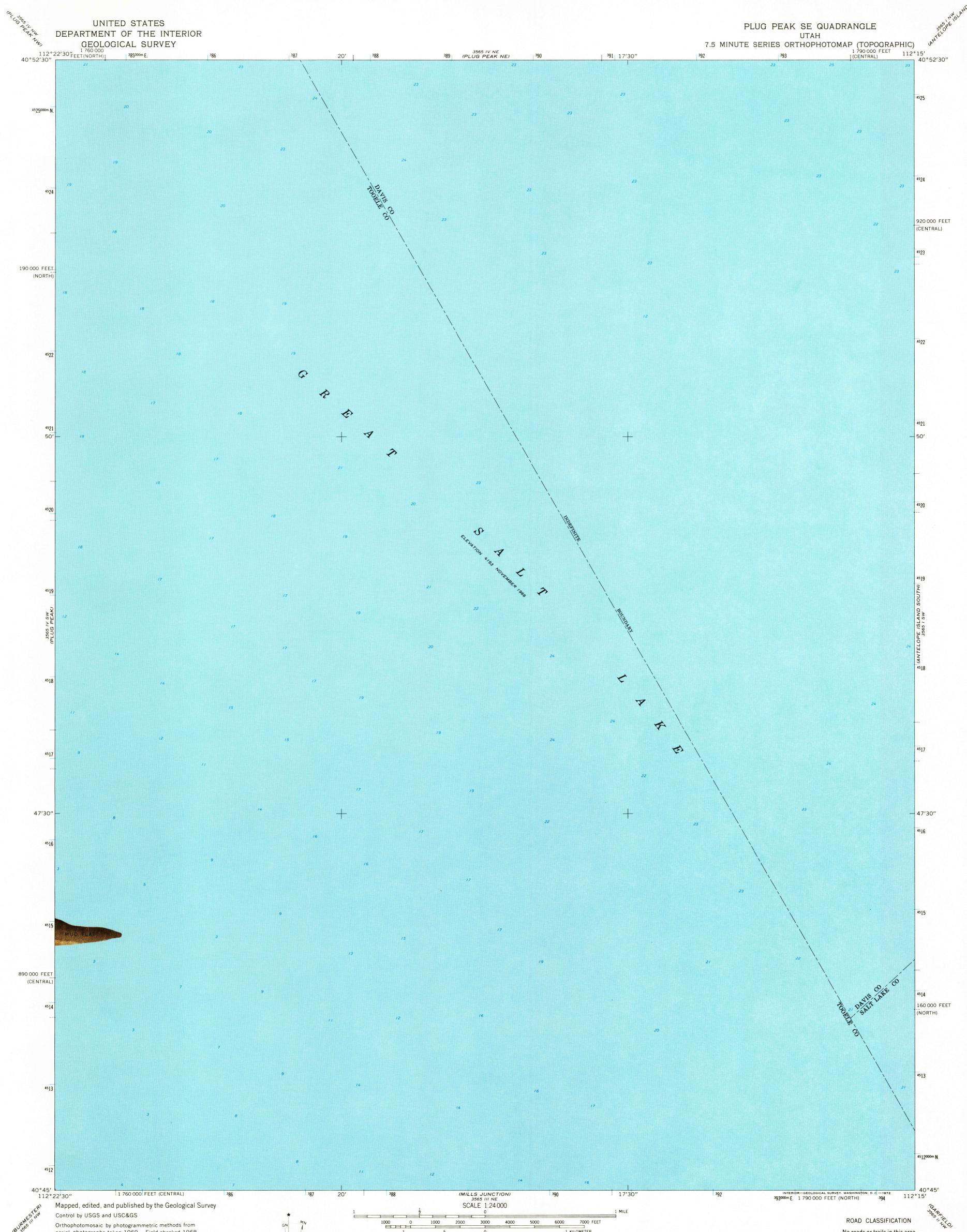
Orthophotomosaic by photogrammetric methods from aerial photographs taken 1969. Field checked 1968 Soundings compiled from chart furnished by U.S. Naval Reserve and information furnished by U.S. Corps of Engineers and Utah Geological and Mineralogical Survey Polyconic projection. 1927 North American datum 10,000-foot grids based on Utah coordinate system, central and north zones 1000-meter Universal Transverse Mercator grid ticks, zone 12, shown in blue
