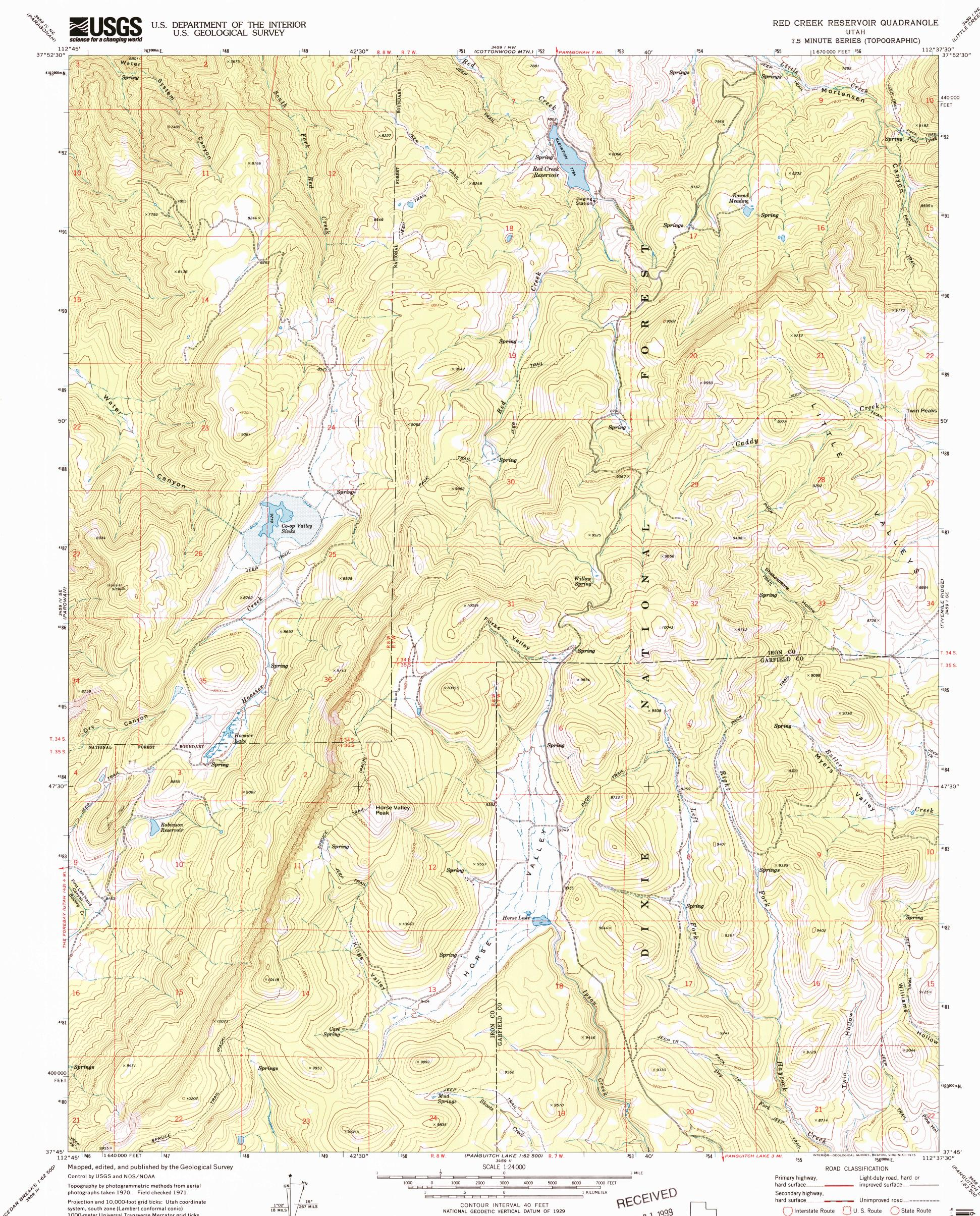
Projection and 10,000-foot grid ticks: Utah coordinate system, south zone (Lambert conformal conic) 1000-meter Universal Transverse Mercator grid ticks, zone 12, shown in blue. 1927 North American datum
