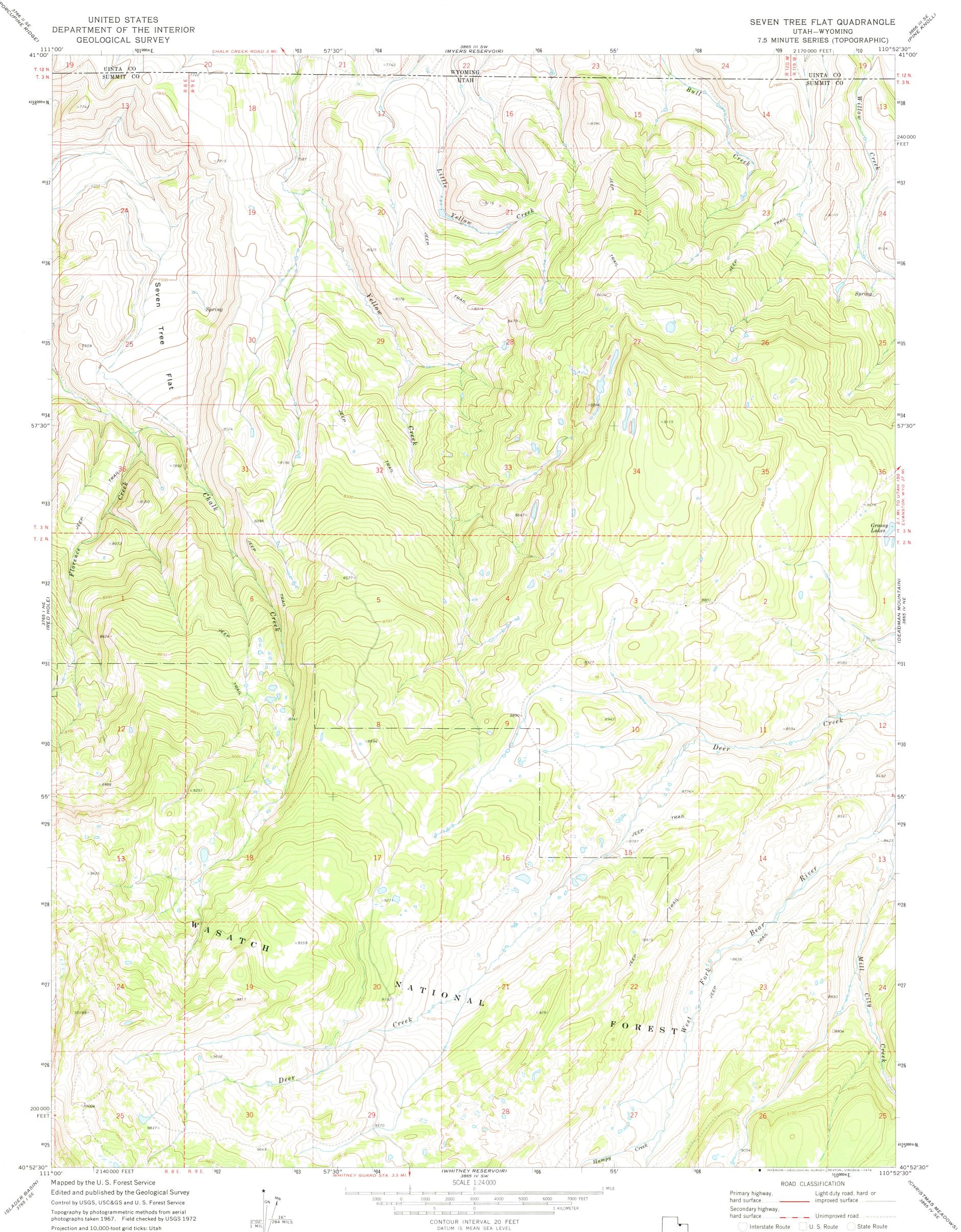
Projection and 10,000-foot grid ticks: Utah coordinate system, north zone (Lambert conformal conic) 1000-meter Universal Transverse Mercator grid ticks, zone 12, shown in blue. 1927 North American datum
