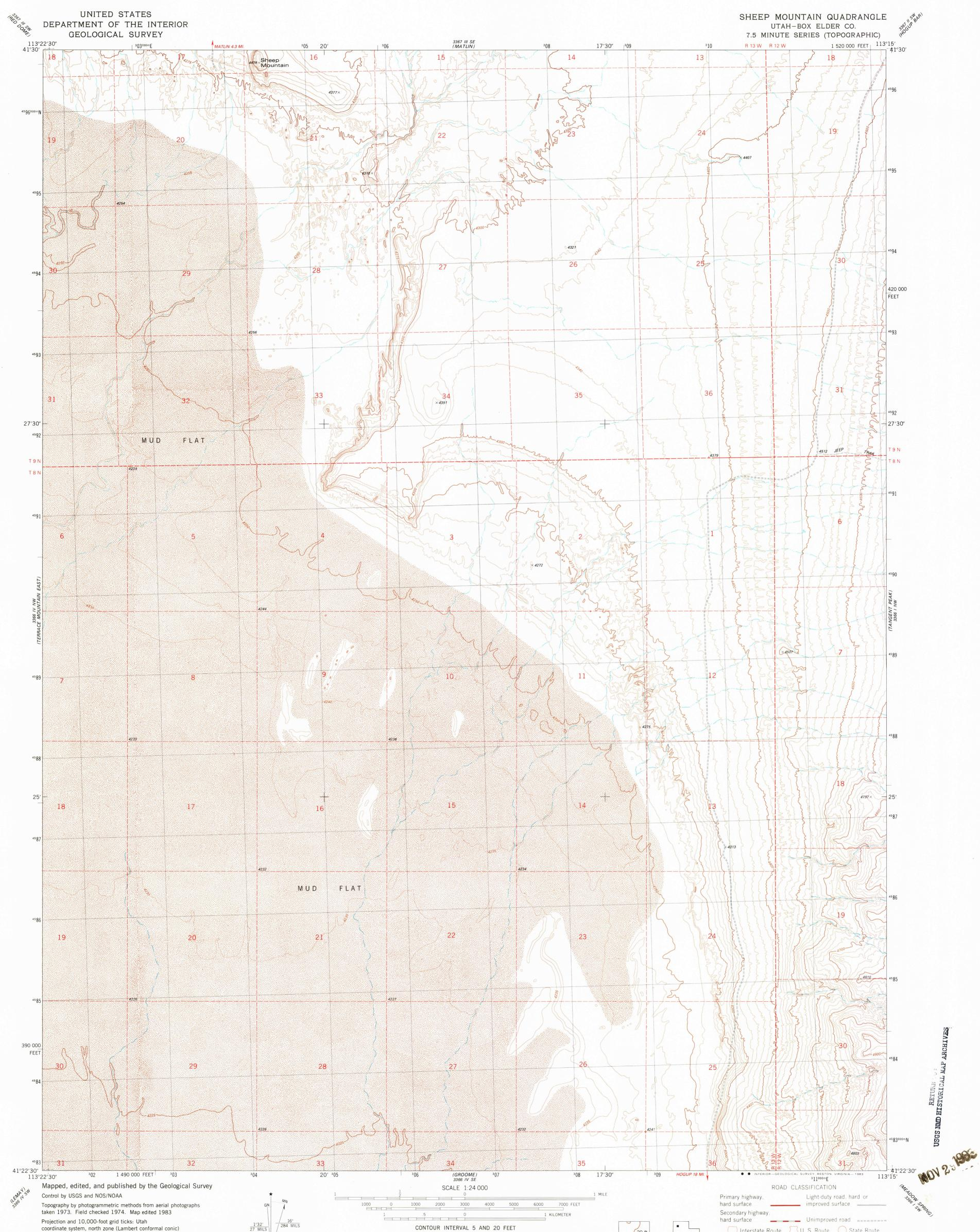
coordinate system, north zone (Lambert conformal conic) 1000-meter Universal Transverse Mercator grid, zone 12 1927 North American datum To place on the predicted North American Datum 1983 move the projection lines 12 meters north and 69 meters east as shown by dashed corner ticks
