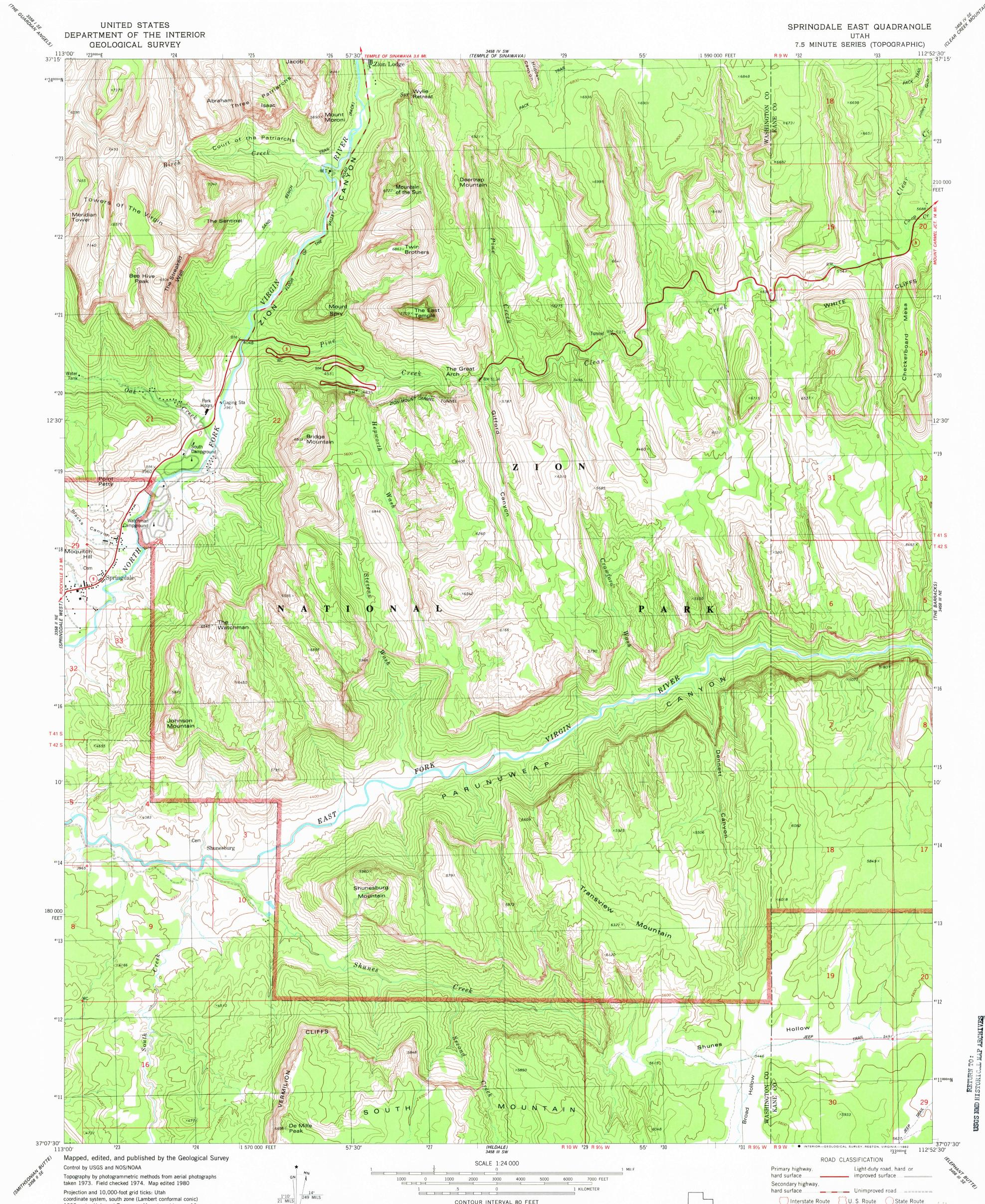
coordinate system, south zone (Lambert conformal conic) 1000-meter Universal Transverse Mercator grid, zone 12 1927 North American datum To place on the predicted North American Datum 1983 move the projection lines 6 meters north and 68 meters east as shown by dashed corner ticks
