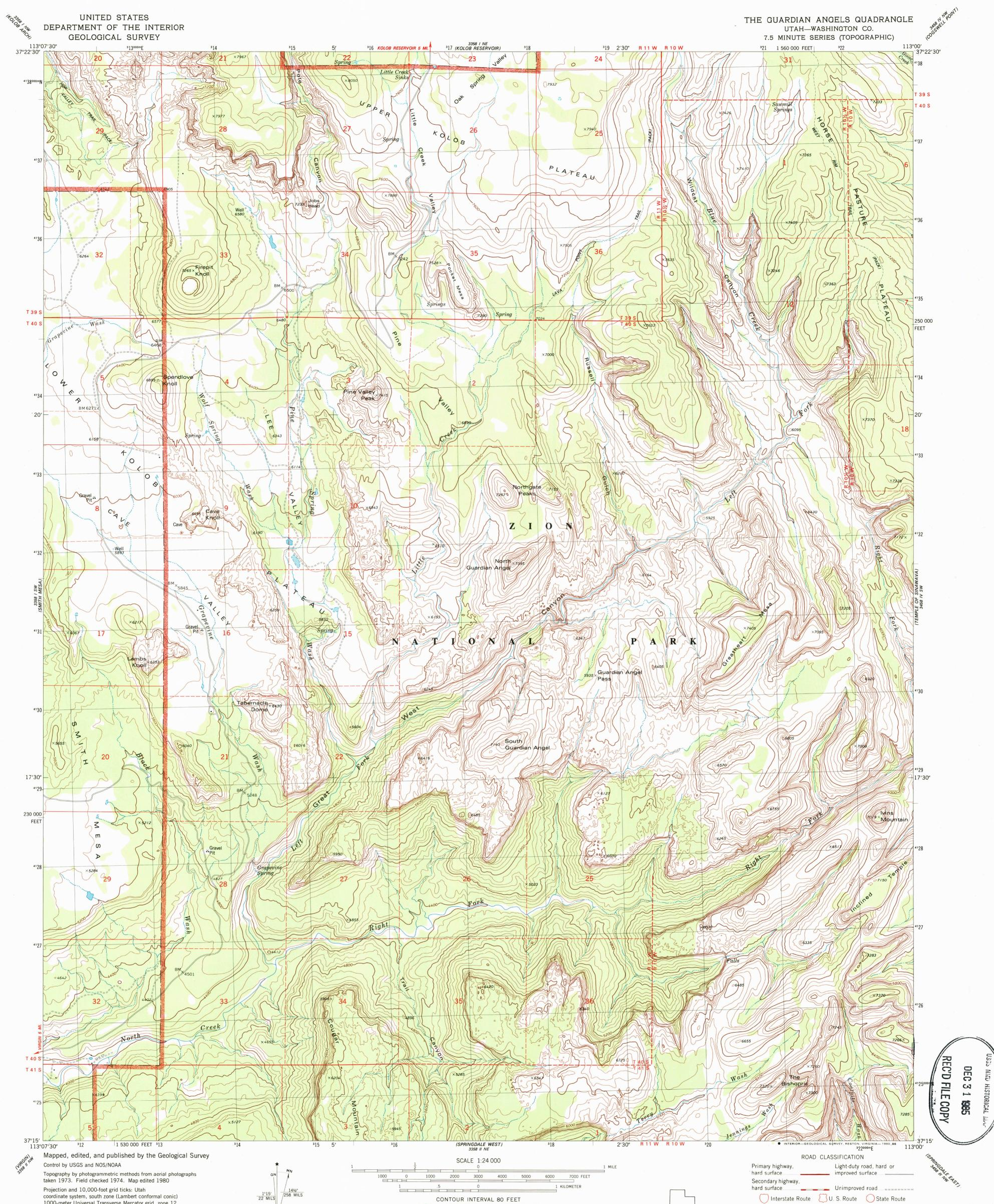
1000-meter Universal Transverse Mercator grid, zone 12 1927 North American datum To place on the predicted North American Datum 1983 move the projection lines 6 meters north and 69 meters east as shown by dashed corner ticks
