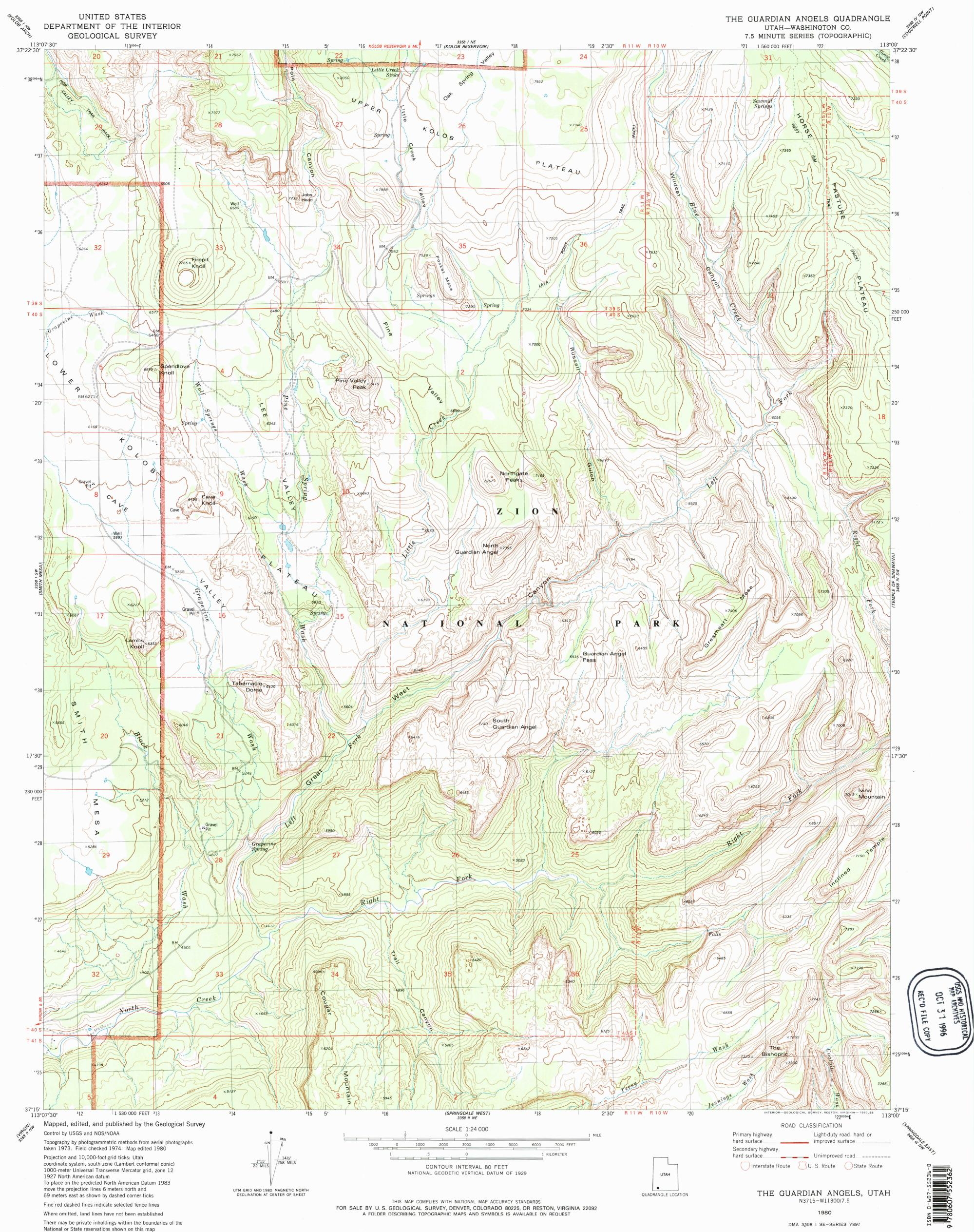
1000-meter Universal Transverse Mercator grid, zone 12 1927 North American datum To place on the predicted North American Datum 1983 move the projection lines 6 meters north and 69 meters east as shown by dashed corner ticks
