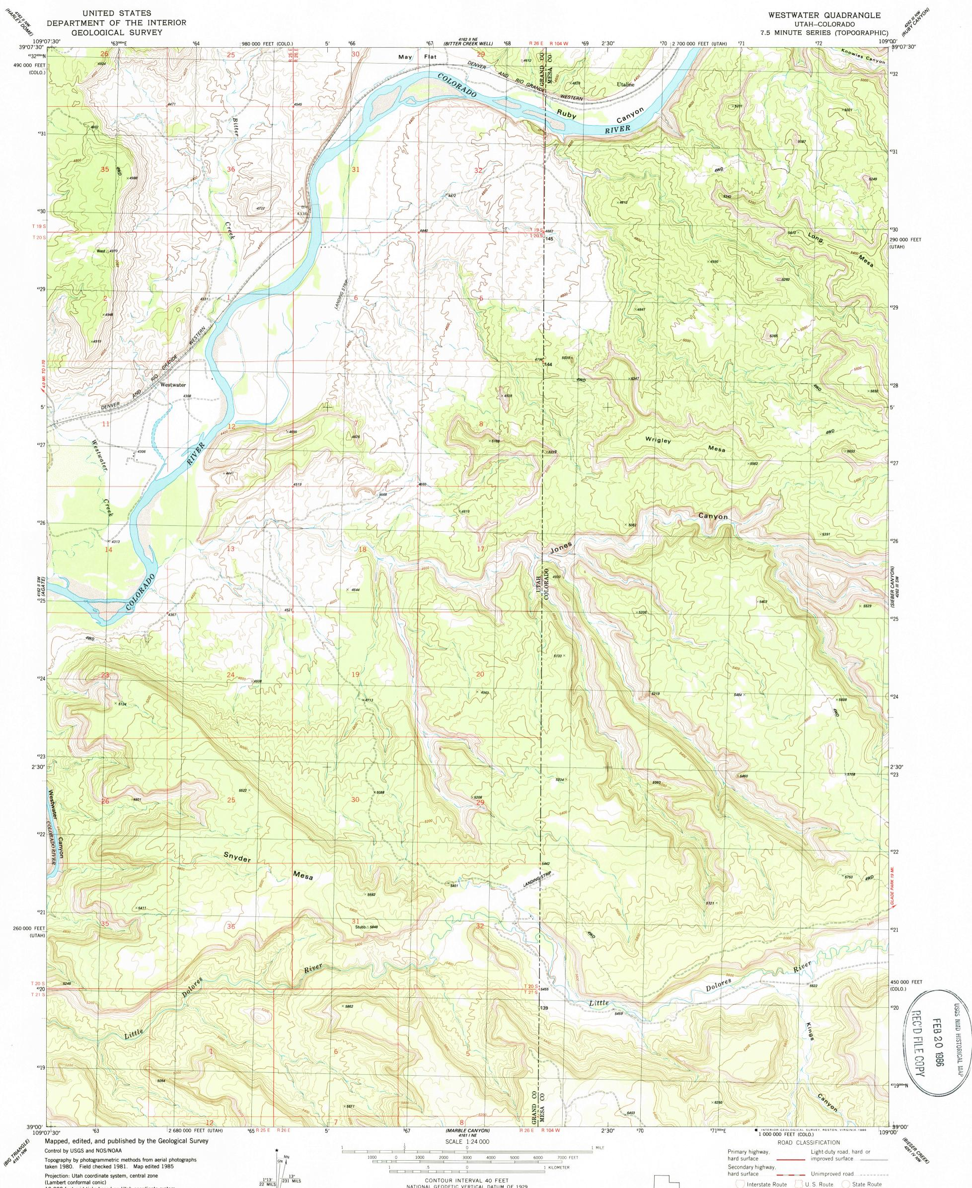
(Lambert conformal conic) 10,000-foot grid ticks based on Utah coordinate system, central zone and Colorado coordinate system, central zone 1000-meter Universal Transverse Mercator grid, zone 12 1927 North American Datum To place on the predicted North American Datum 1983 move the projection lines 6 meters north and 58 meters east as shown by dashed corner ticks
