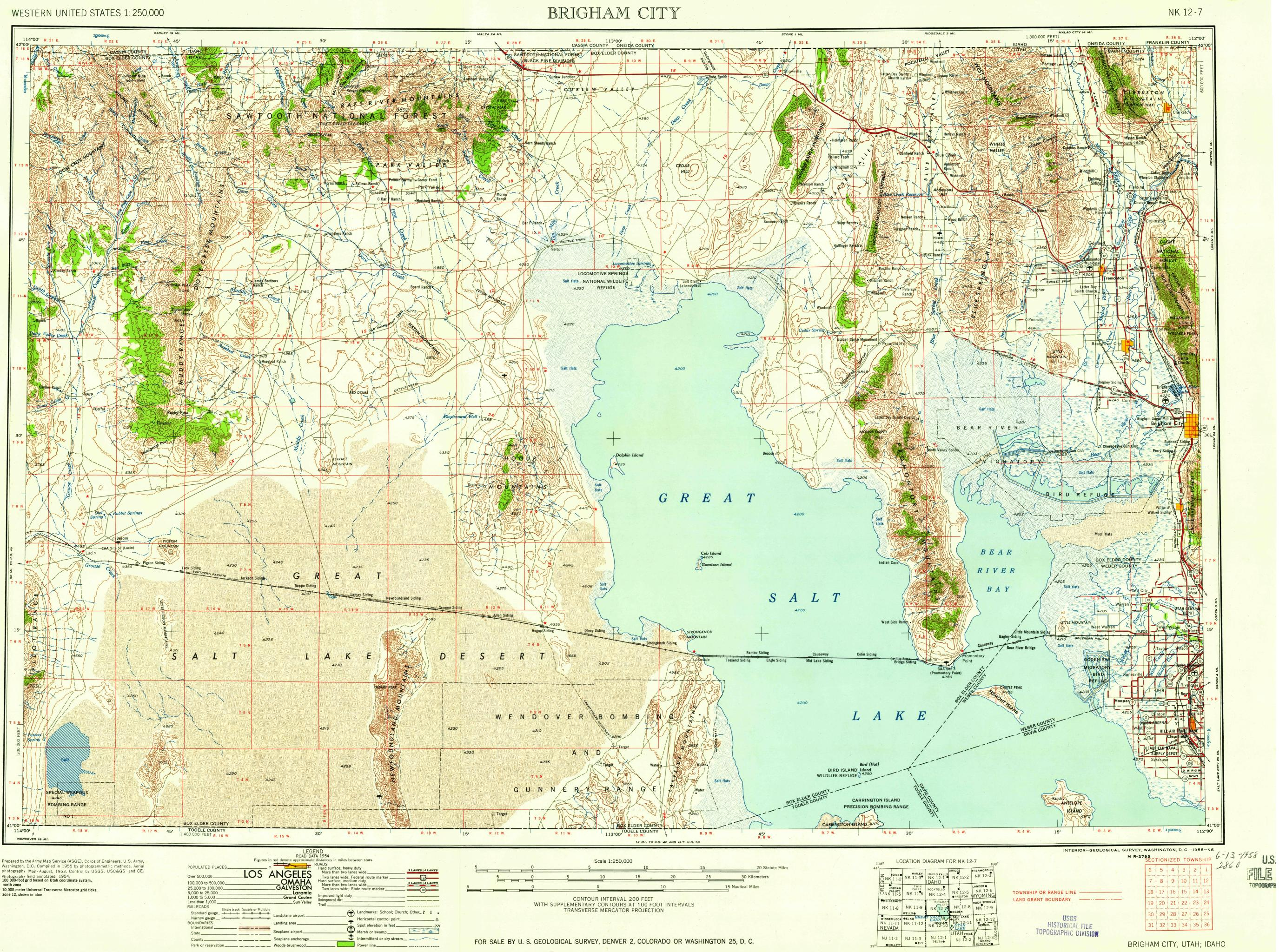
Prepared by the Army Map Service (ASGE), Corps of Engineers, U.S. Army, Washington, D.C. Compiled in 1955 by photogrammetric methods. Aerial photography May - August, 1953. Control by USGS, USC&GS and CE. Photography field annotated 1954. 100,000-foot grid based on Utah coordinate system, arth actions and north zone 10,000-meter Universal Transverse Mercator grid ticks,
