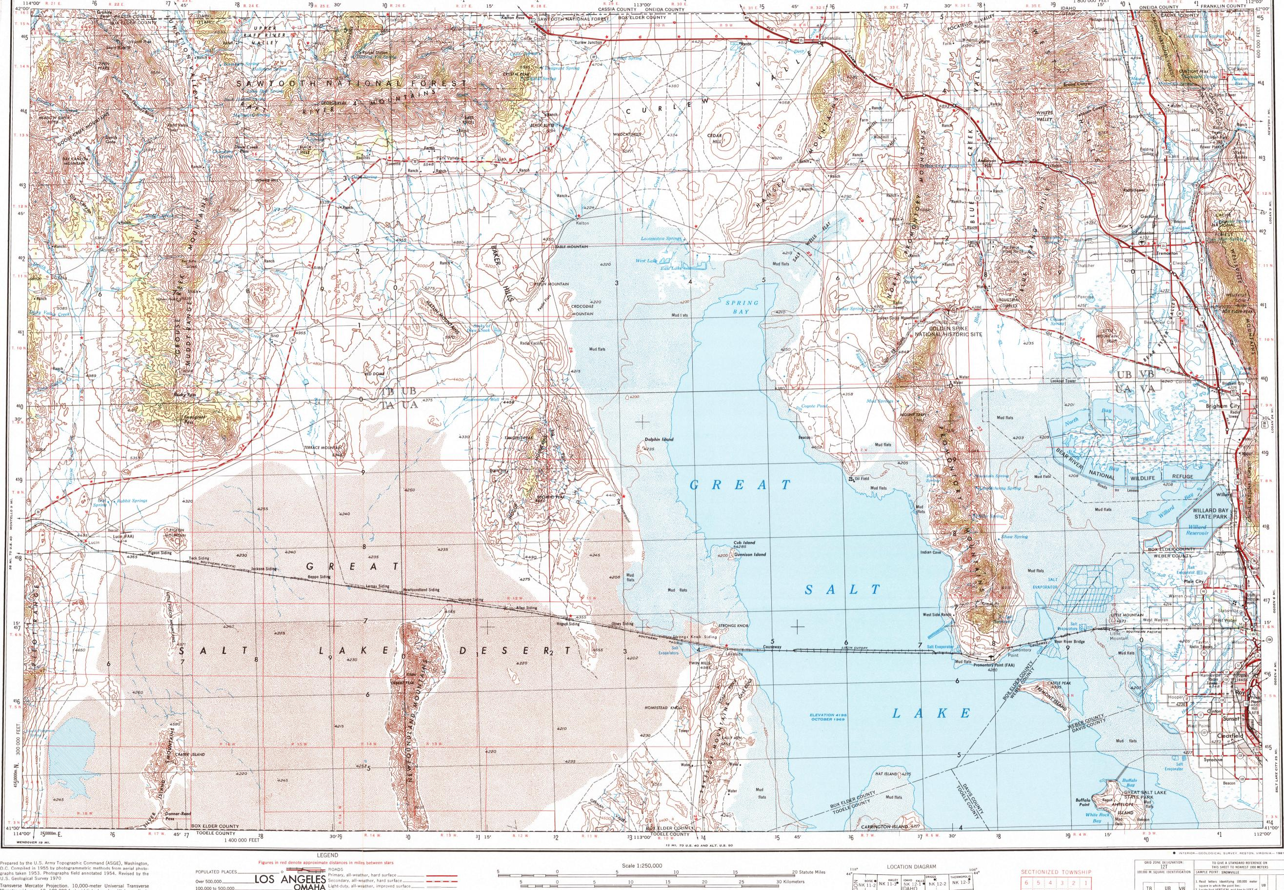
Prepared by the U.S. Army Topographic Command (ASGE), Washington, D.C. Compiled in 1955 by photogrammetric methods from aerial photographs taken 1953. Photographs field annotated 1954. Revised by the
