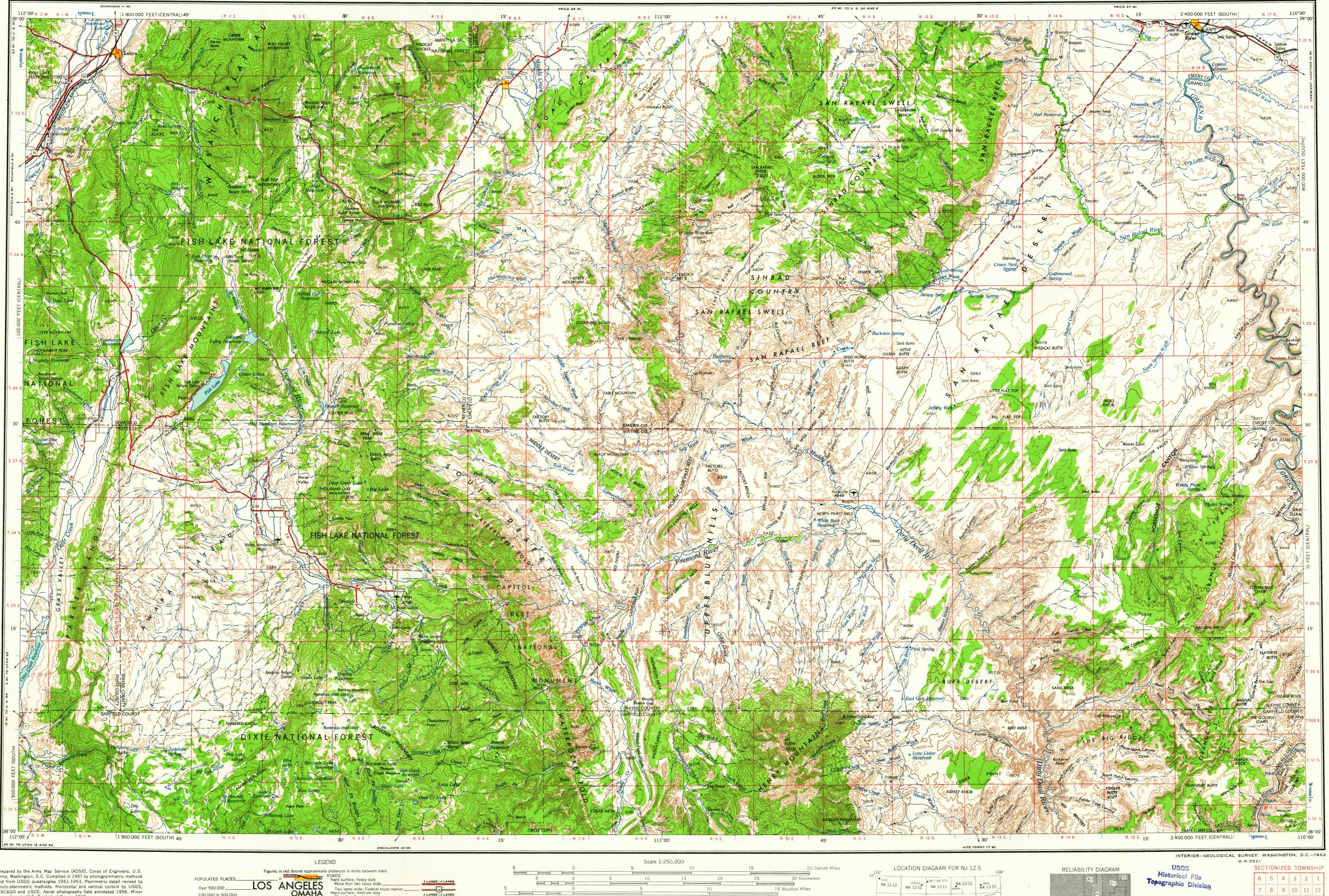
Prepared by the Army Map Service (AOSX), Corps of Engineers, U.S. Army, Washington, D.C. Compiled in 1957 by photogrammetric methods and from USGS quadrangles 1951-1953. Planimetric detail revised by photo-planimetric methods. Horizontal and vertical control by USGS, USC&GS and USCE. Aerial photography field annotated 1956. Minor corrections by U.S. Geological Survey 1962.
