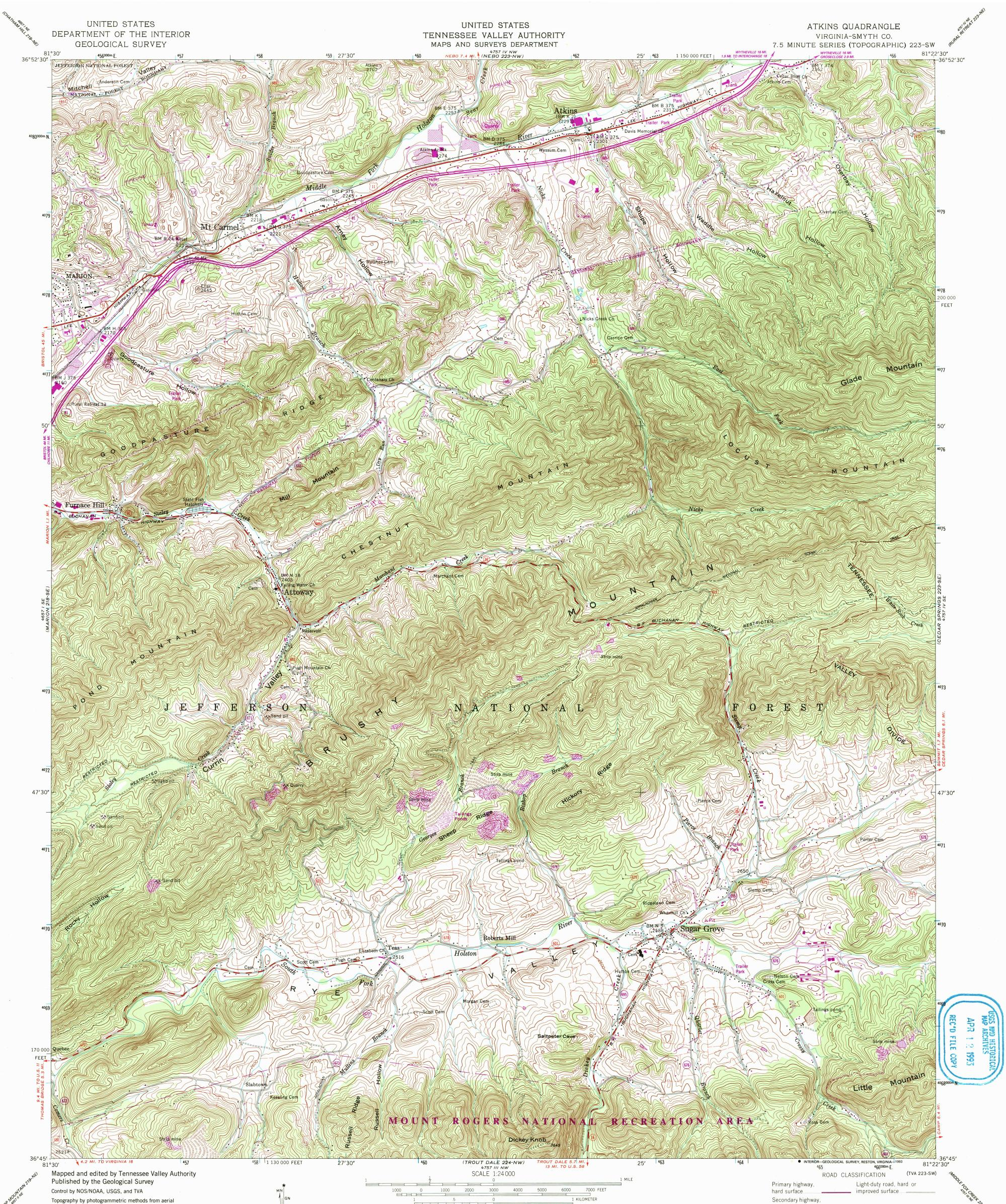
photographs taken 1948. Field checked by TVA 1958 Polyconic projection. 1927 North American Datum 10,000-foot grid ticks based on Virginia coordinate system, south zone 1000-meter Universal Transverse Mercator grid ticks, zone 17, shown in blue To place on the predicted North American Datum 1983 move the projection lines 8 meters south and 15 meters west as shown by dashed corner ticks Fine red dashed lines indicate selected fence and field lines where
