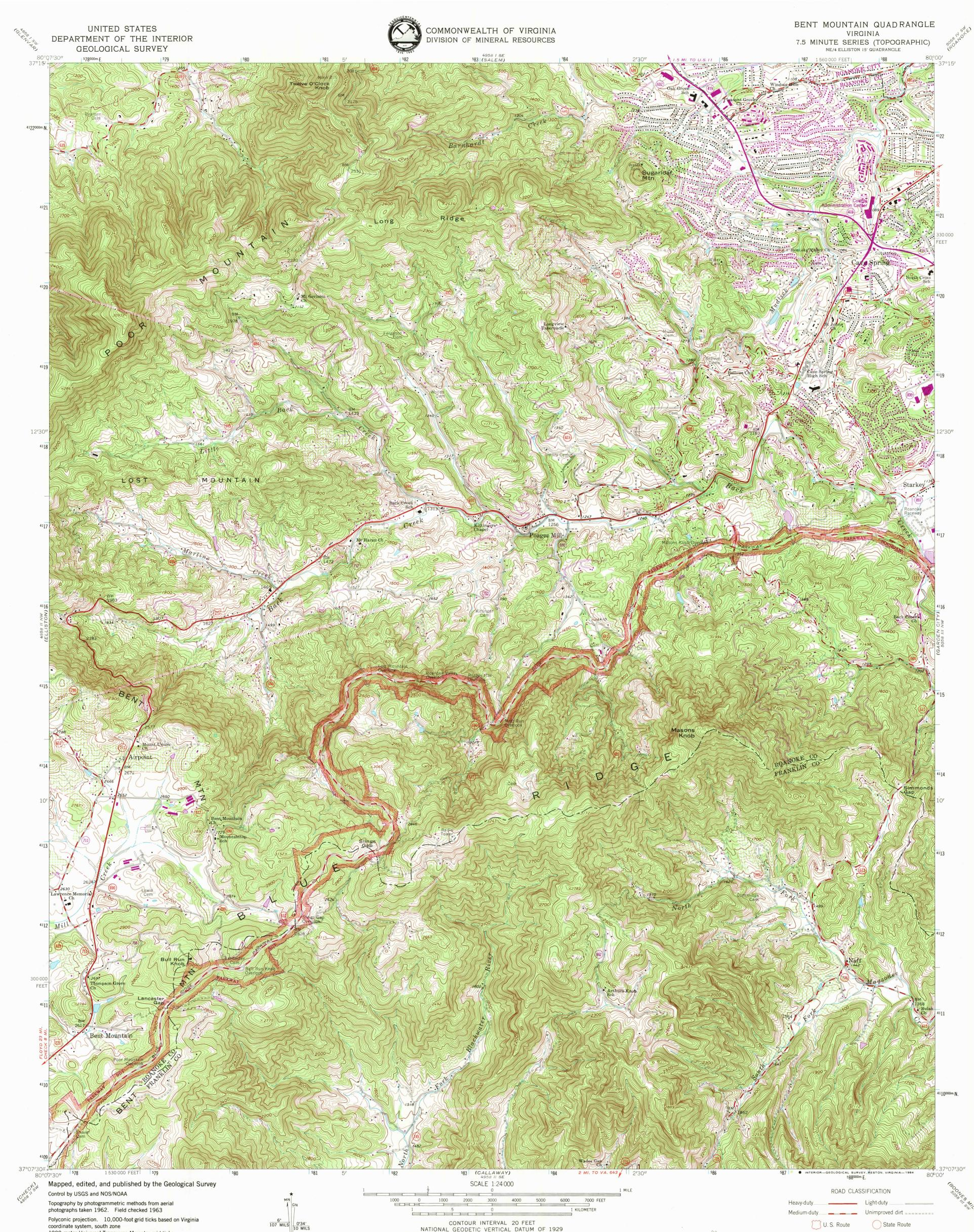
Polyconic projection. 10,000-foot grid ticks based on Virginia coordinate system, south zone 1000-meter Universal Transverse Mercator grid ticks, zone 17, shown in blue 1927 North American Datum To place on the predicted North American Datum 1983 move the projection lines 9 meters south and 19 meters west as shown by dashed corner ticks Fine red dashed lines indicate selected fence and field lines where
