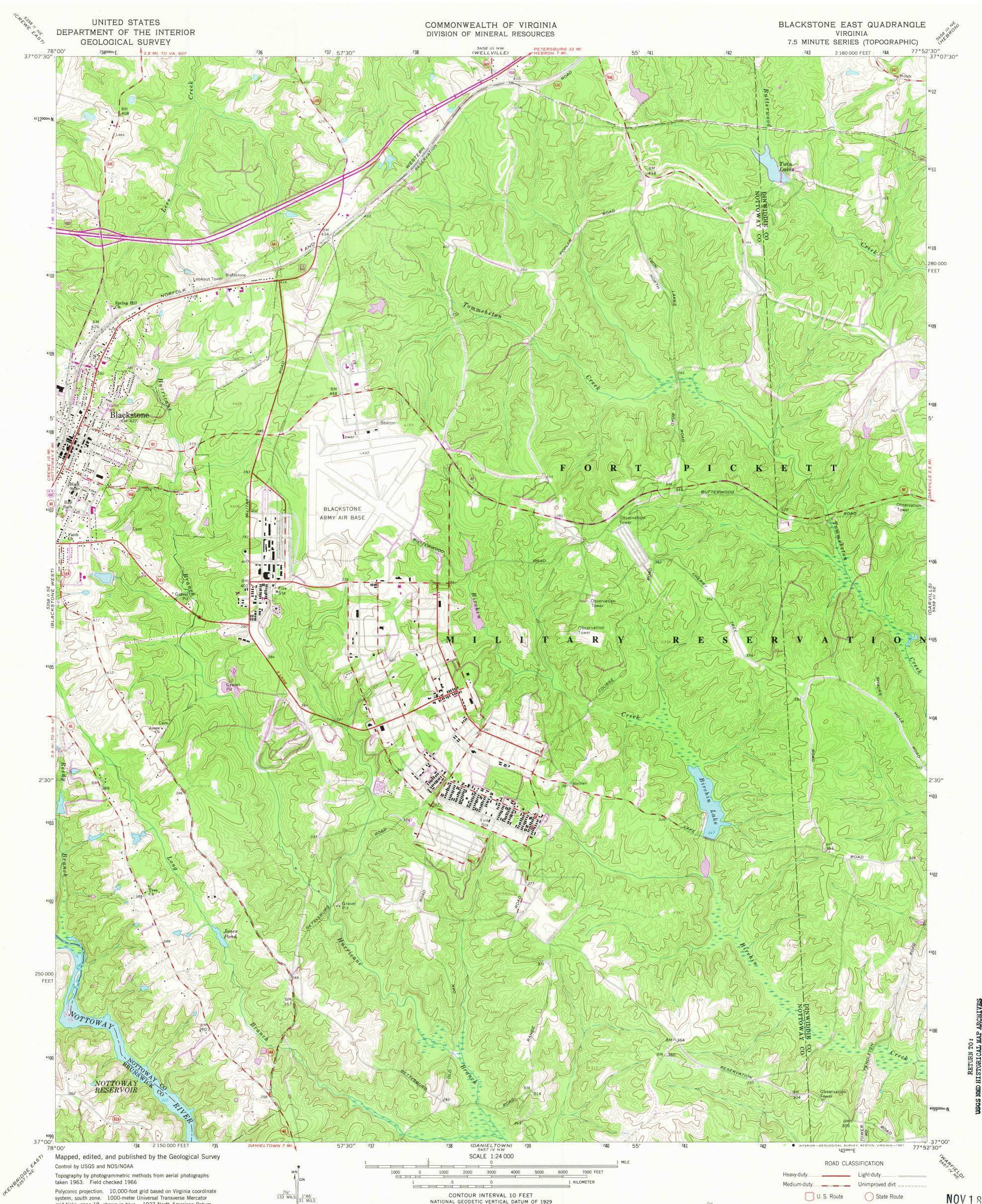
system, south zone. 1000-meter Universal Transverse Mercator grid ticks, zone 18, shown in blue. 1927 North American Datum To place on the predicted North American Datum 1983 move the projection lines 12 meters south and 26 meters west as shown by dashed corner ticks
