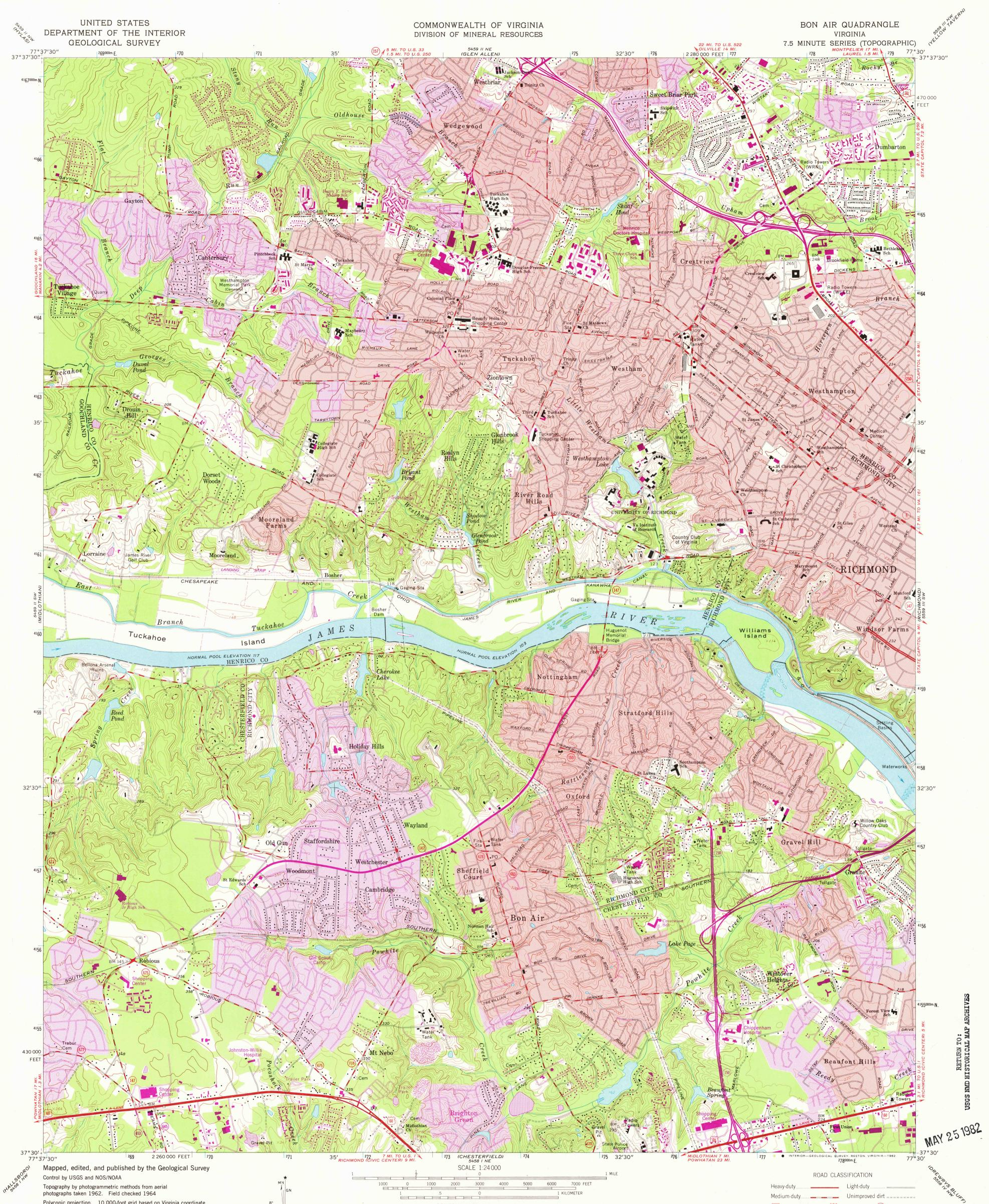
Polyconic projection. 10,000-foot grid based on Virginia coordinate system, south zone. 1000-meter Universal Transverse Mercator grid ticks, zone 18, shown in blue. 1927 North American Datum To place on the predicted North American Datum 1983 move the projection lines 11 meters south and 26 meters west as shown by dashed corner ticks
