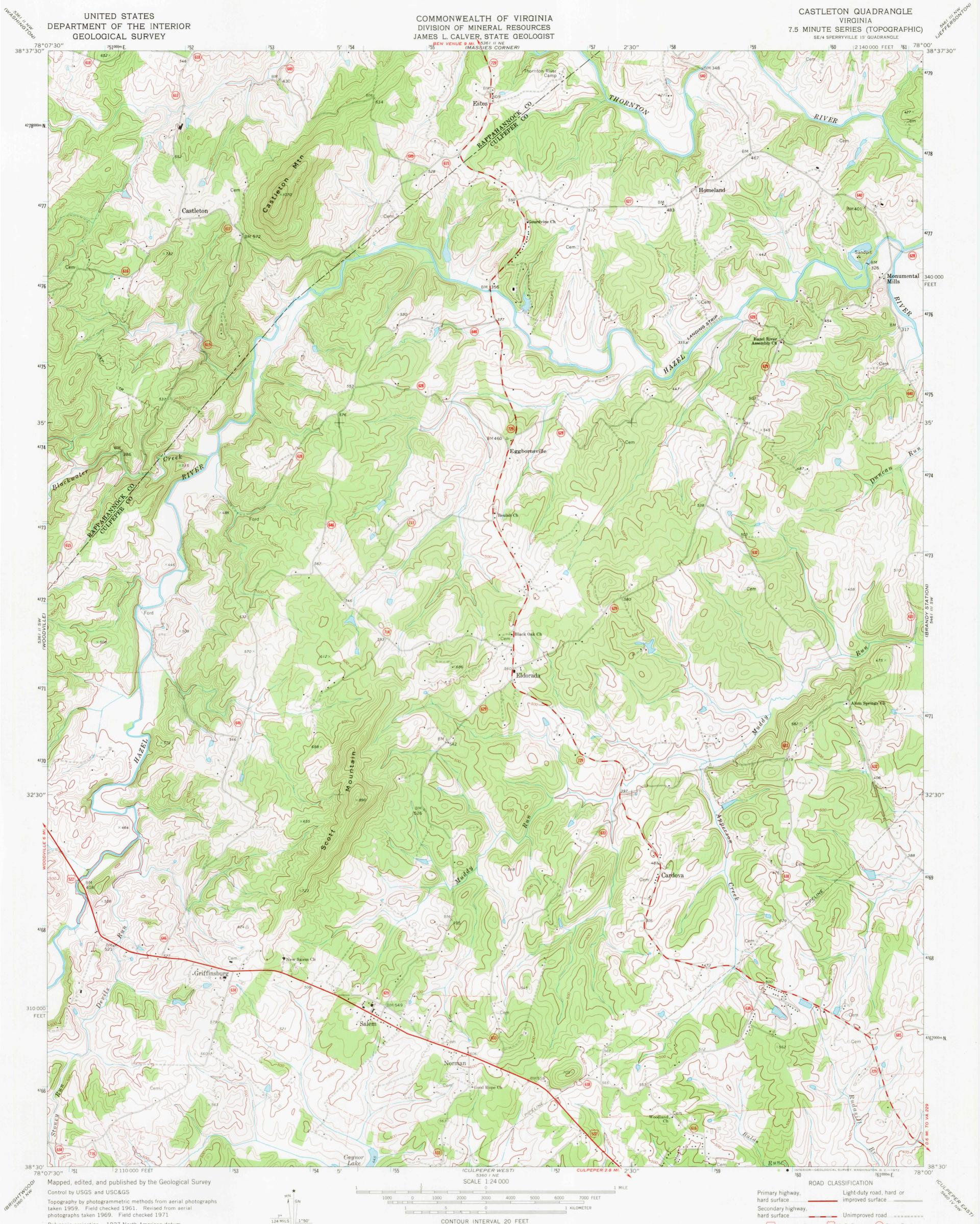
Polyconic projection. 1927 North American datum 10,000-foot grid based on Virginia coordinate system, north zone 1000-meter Universal Transverse Mercator grid ticks, zone 17, shown in blue Fine red dashed lines indicate selected fence and field lines where
