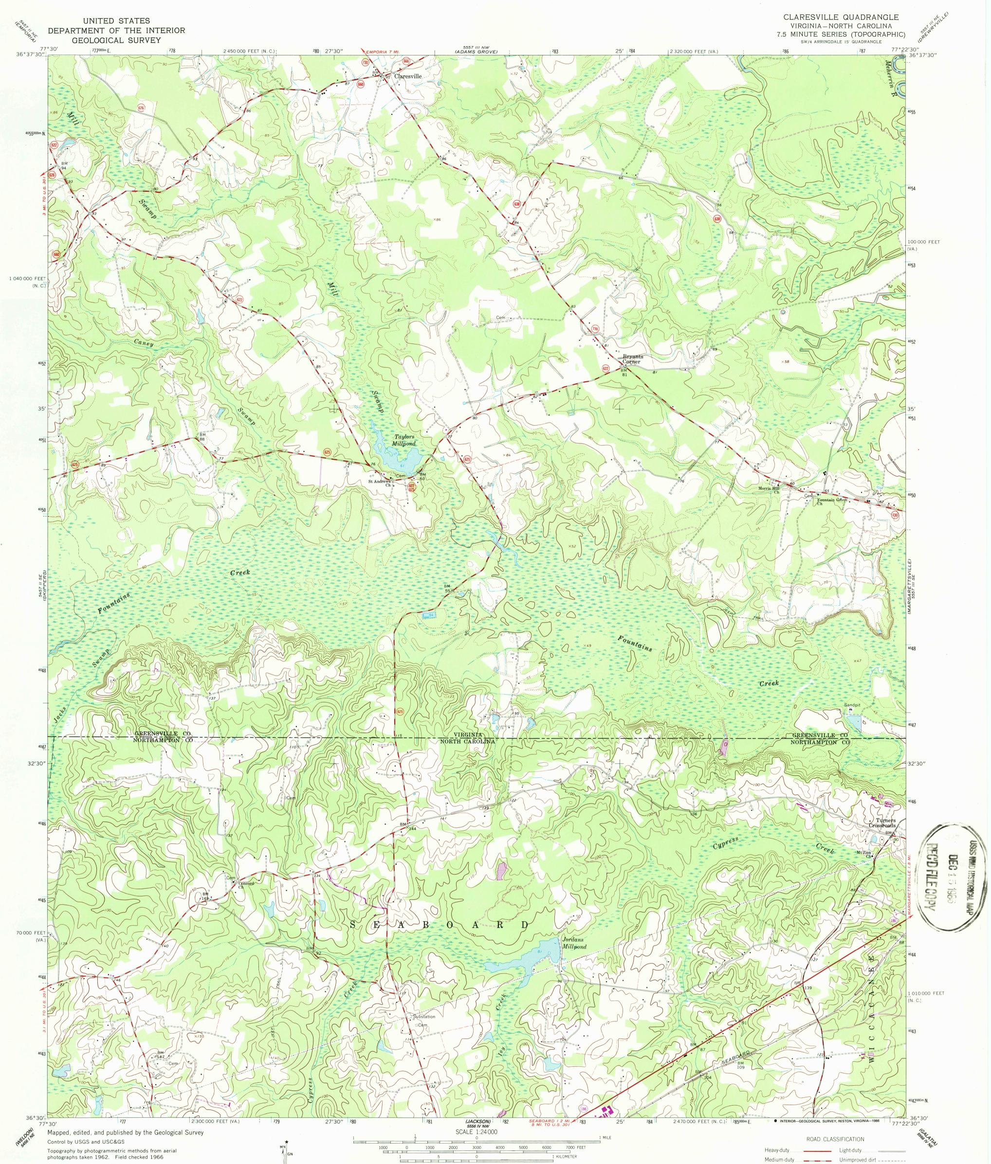
Polyconic projection. 1927 North American datum 10,000-foot grids based on Virginia coordinate system, south zone, and North Carolina coordinate system 1000-meter Universal Transverse Mercator grid ticks, zone 18 shown in blue
