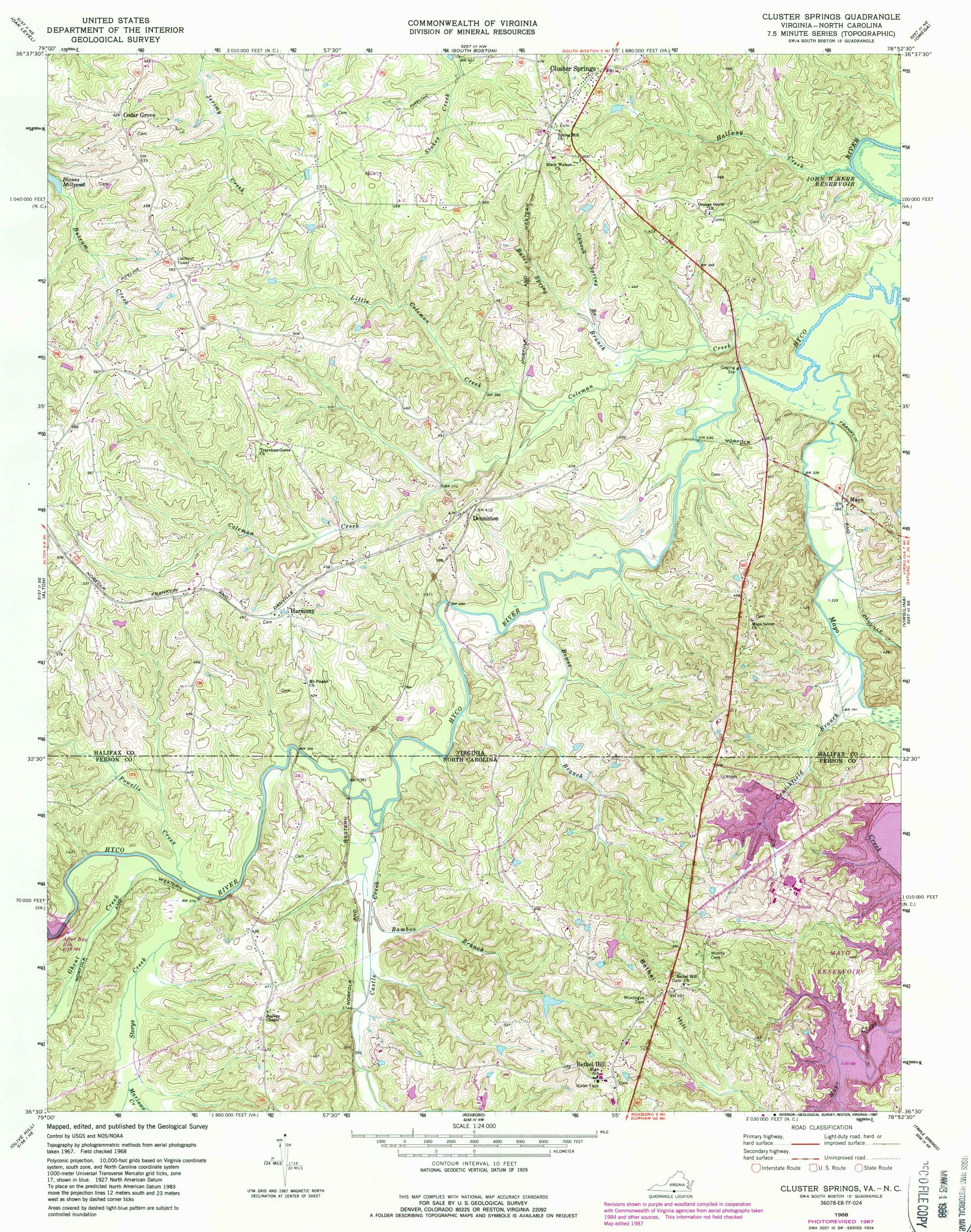
Polyconic projection. 10,000-foot grids based on Virginia coordinate system, south zone, and North Carolina coordinate system 1000-meter Universal Transverse Mercator grid ticks, zone 17, shown in blue. 1927 North American Datum To place on the predicted North American Datum 1983 move the projection lines 12 meters south and 23 meters west as shown by dashed corner ticks
