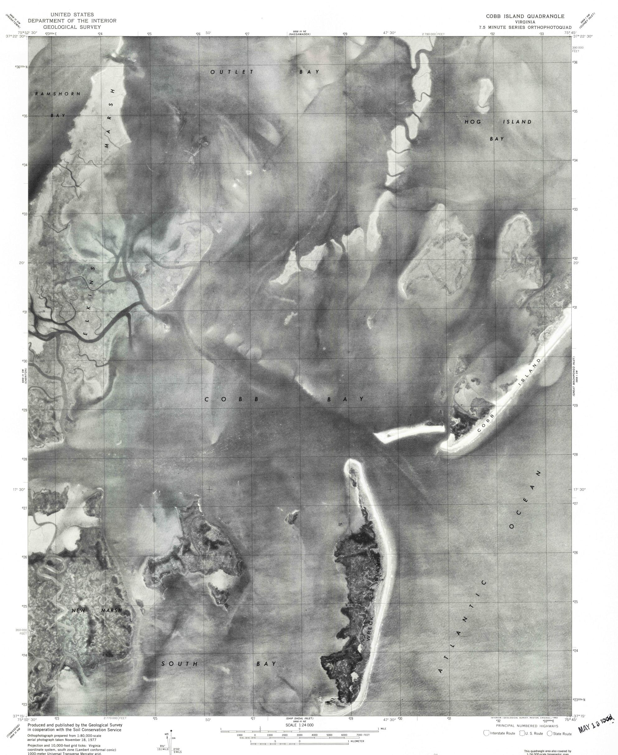
Projection and 10,000-foot grid ticks: Virginia coordinate system, south zone (Lambert conformal conic) 1000-meter Universal Transverse Mercator grid, zone 18. 1927 North American Datum
