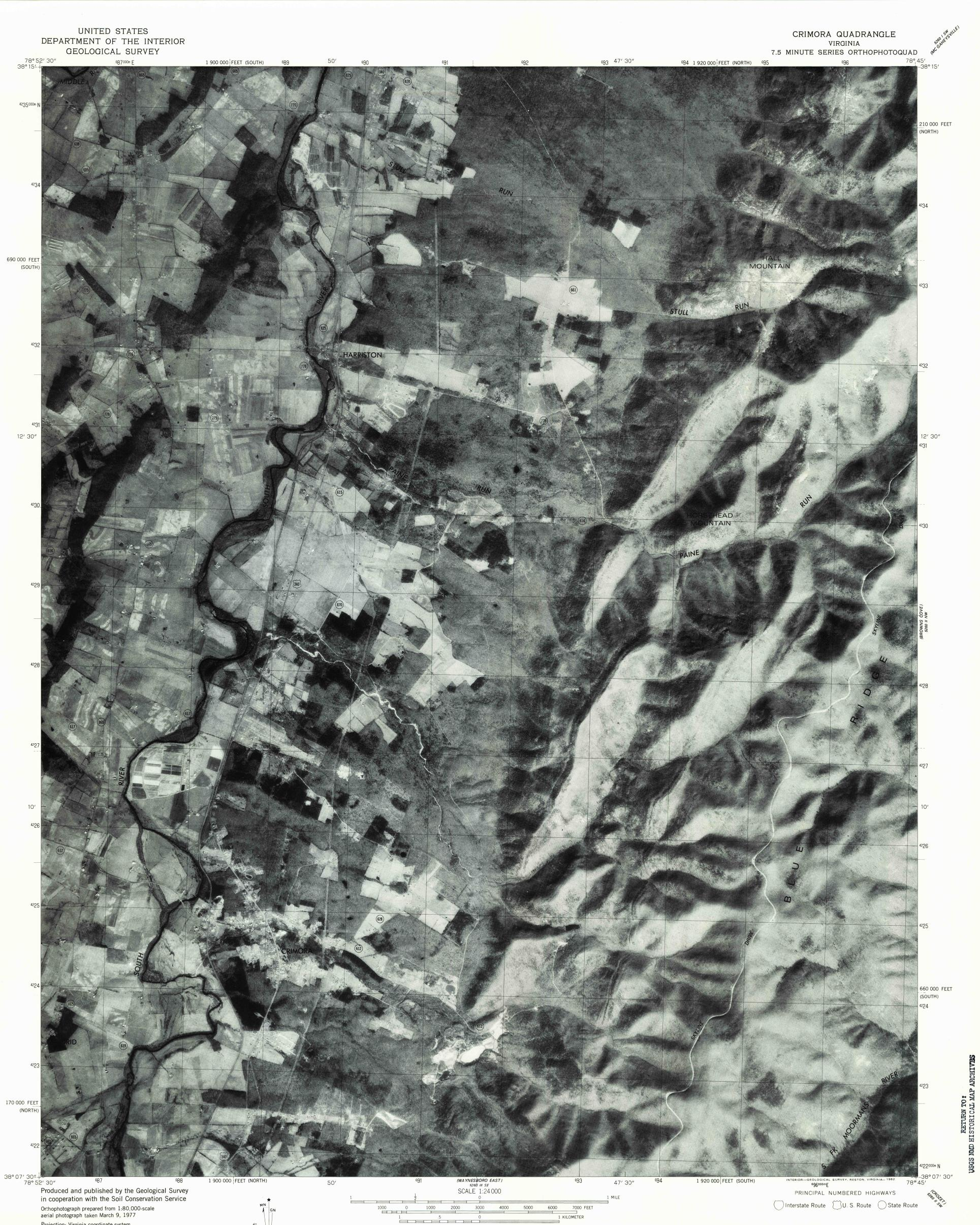
Projection: Virginia coordinate system, north zone (Lambert conformal conic) 10,000-foot grid ticks based on Virginia coordinate system, north and south zones 1000-meter Universal Transverse Mercator grid, zone 17. 1927 North American Datum
