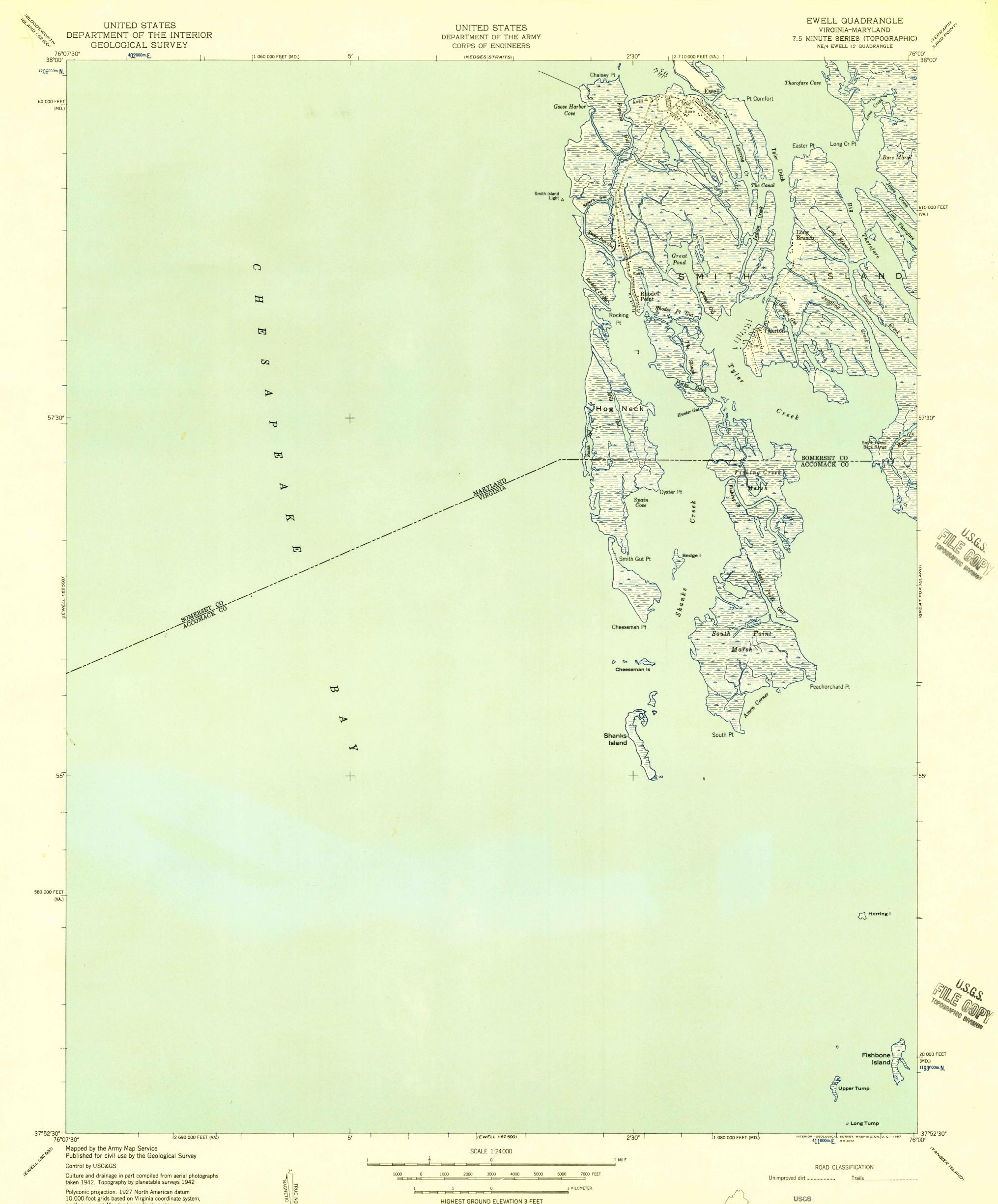
Polyconic projection. 1927 North American datum 10,000-foot grids based on Virginia coordinate system, south zone, and Maryland coordinate system 1000-meter Universal Transverse Mercator grid ticks, zone 18, shown in blue
