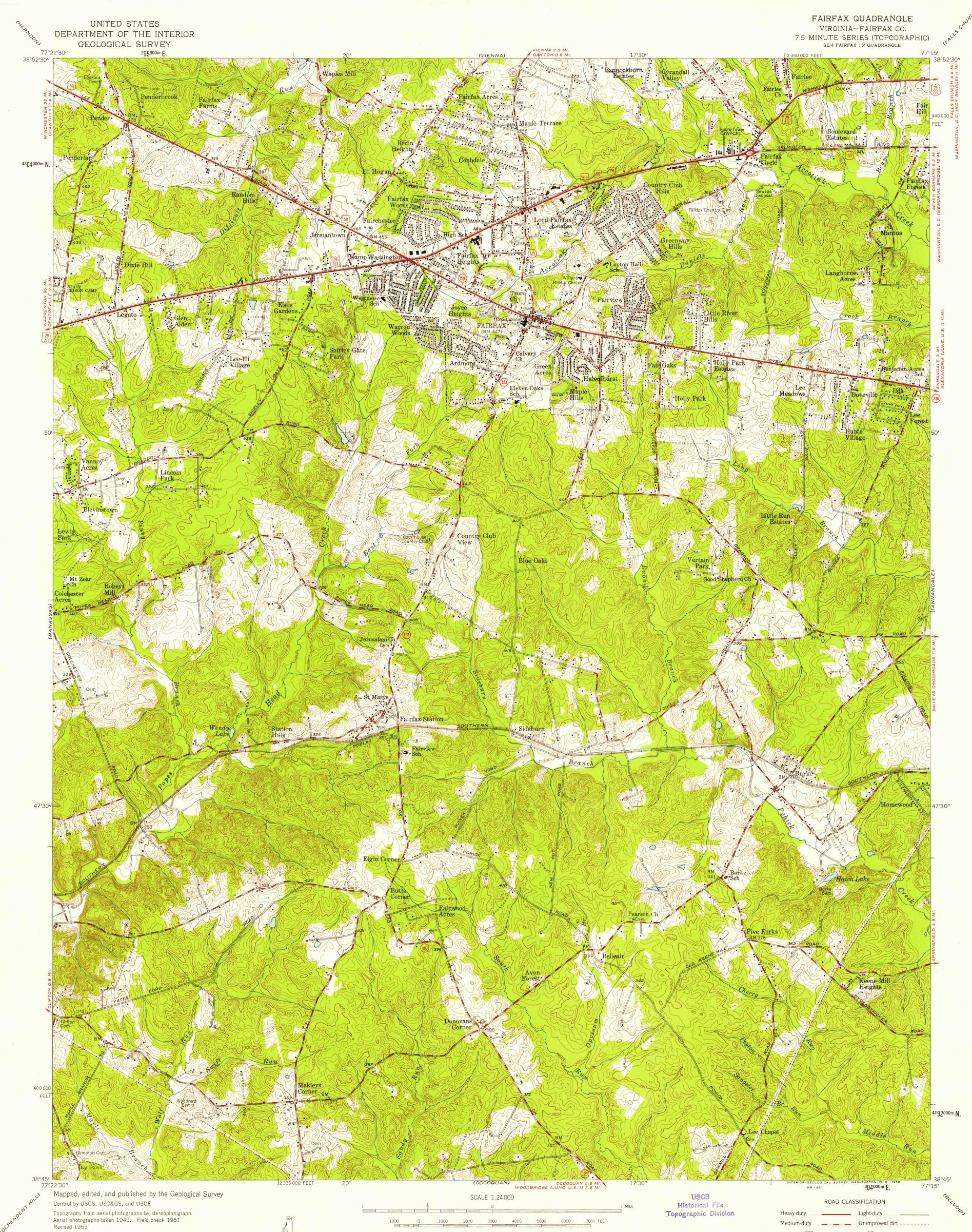
Polyconic projection. 1927 North American datum 10,000-foot grid based on Virginia coordinate system, north zone. 1000-meter Universal Transverse Mercator grid ticks, zone 18, shown in blue
