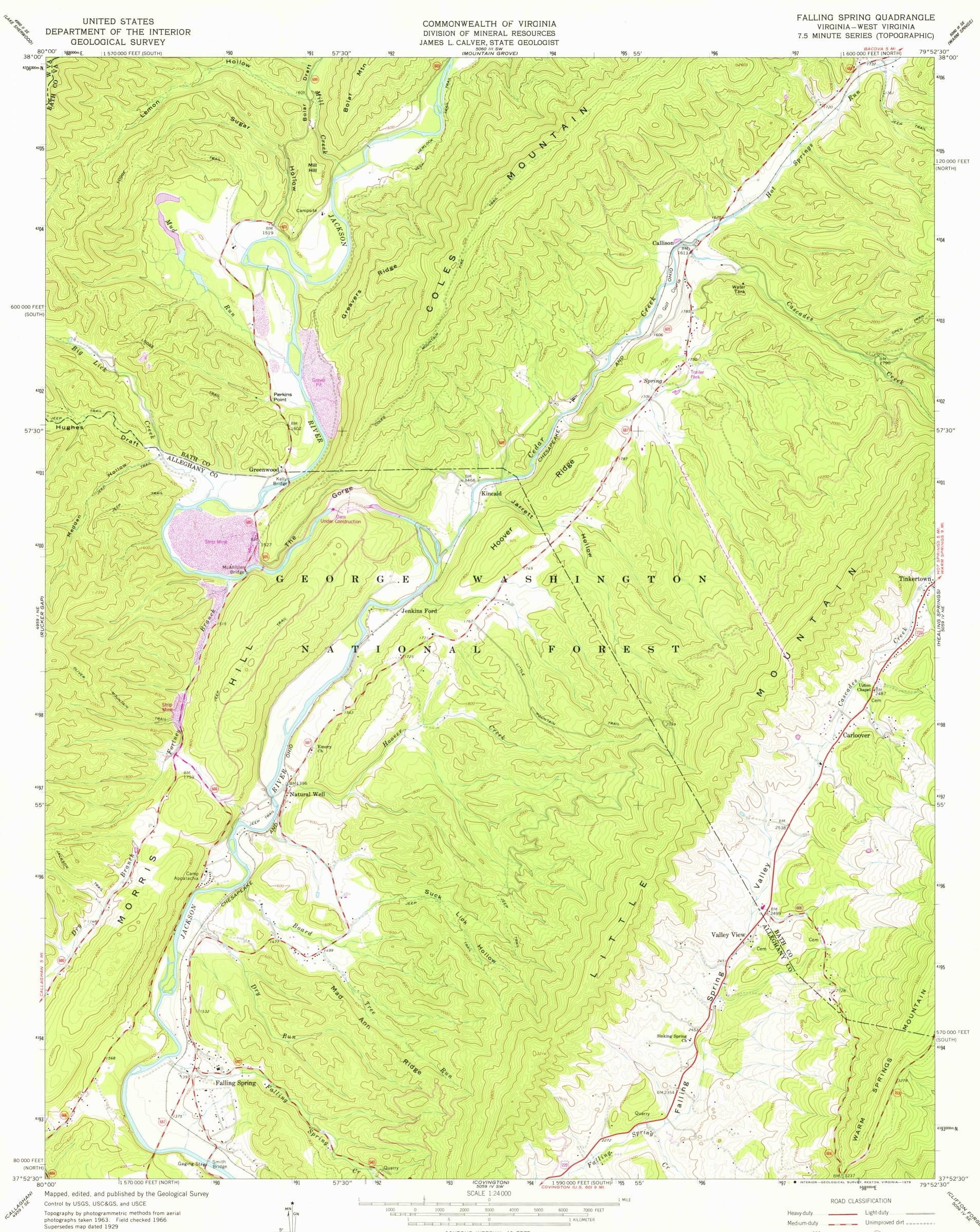
Polyconic projection. 1927 North American datum 10,000-foot grids based on Virginia coordinate system, north and south zones 1000-meter Universal Transverse Mercator grid ticks, zone 17, shown in blue
