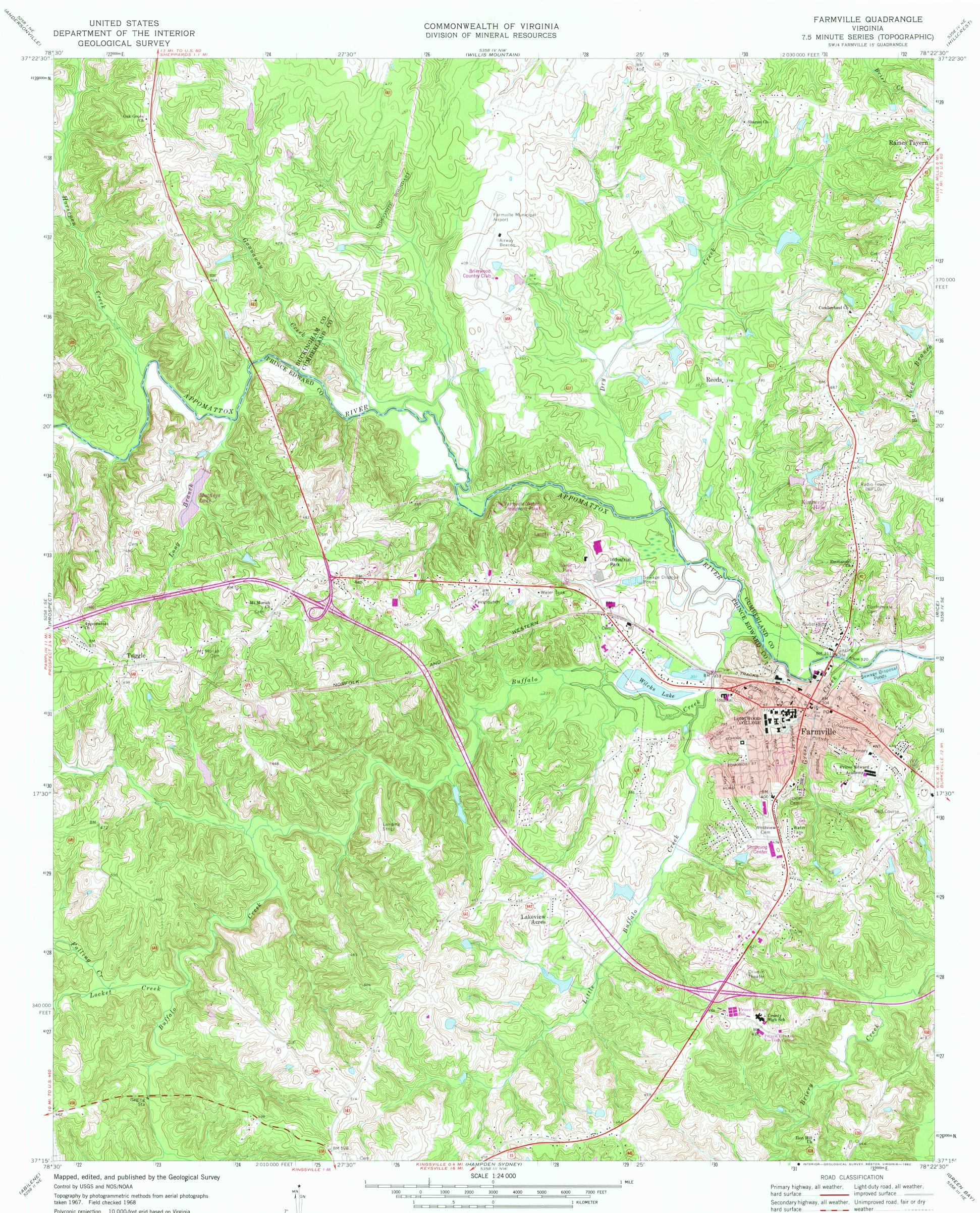
Polyconic projection. 10,000-foot grid based on Virginia coordinate system, south zone. 1000-meter Universal Transverse Mercator grid ticks, zone 17, shown in blue. 1927 North American Datum. To place on the predicted North American Datum 1983 move the projection lines 11 meters south and 24 meters west as shown by dashed corner ticks
