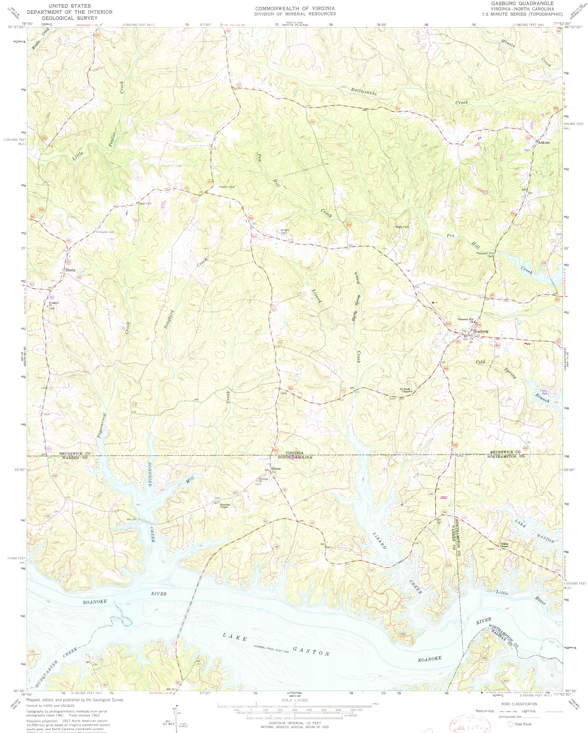
10,000-foot grids based on Virginia coordinate system, south zone, and North Carolina coordinate system 1000-meter Universal Transverse Mercator grid ticks, zone 18, shown in blue
