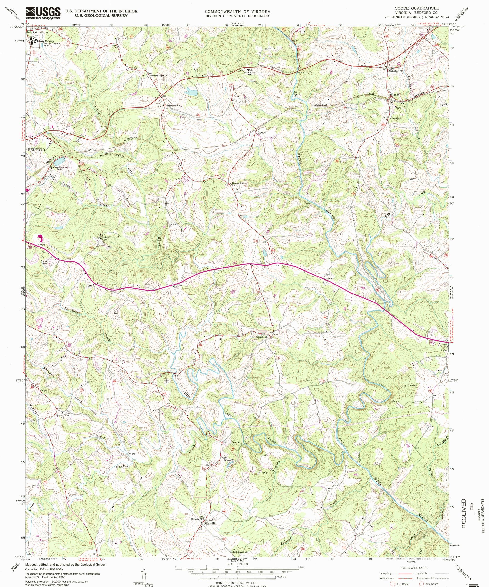
Polyconic projection. 10,000-foot grid ticks based on Virginia coordinate system, south zone 1000-meter Universal Transverse Mercator grid ticks, zone 17, shown in blue 1927 North American Datum To place on the predicted North American Datum 1983 move the projection lines 10 meters south and 21 meters west as shown by dashed corner ticks
