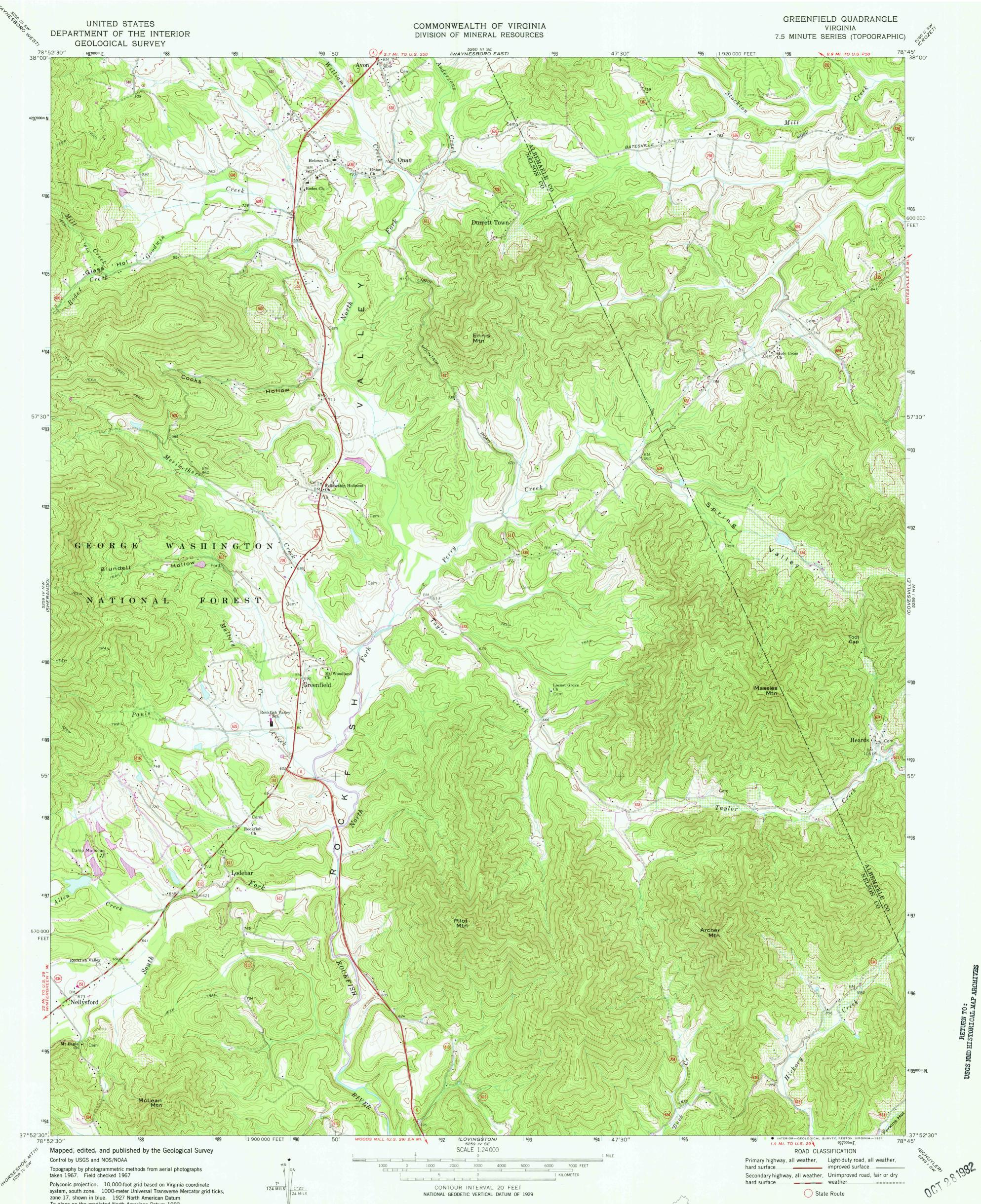
Polyconic projection. 10,000-foot grid based on Virginia coordinate system, south zone. 1000-meter Universal Transverse Mercator grid ticks, zone 17, shown in blue. 1927 North American Datum To place on the predicted North American Datum 1983 move the projection lines 10 meters south and 23 meters west as shown by dashed corner ticks
