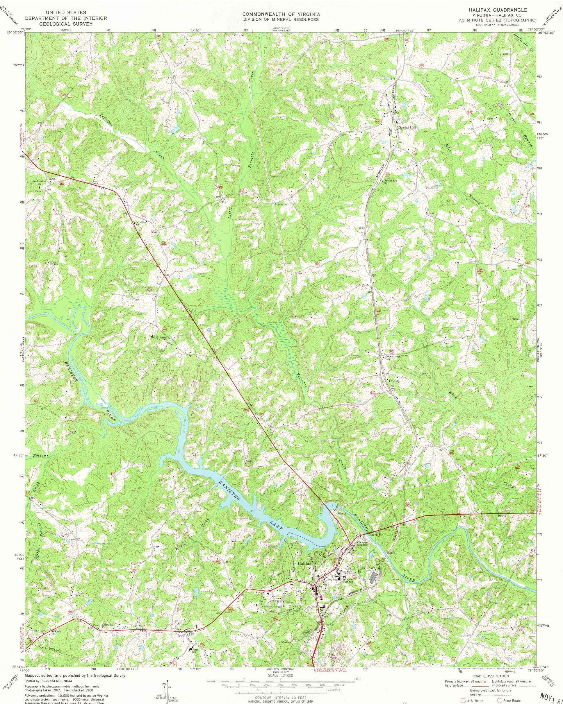
Polyconic projection. 10,000-foot grid based on Virginia coordinate system, south zone. 1000-meter Universal Transverse Mercator grid ticks, zone 17, shown in blue 1927 North American Datum. To place on the predicted North American Datum 1983, move the projection lines 12 meters south and 23 meters west as shown by dashed corner ticks
