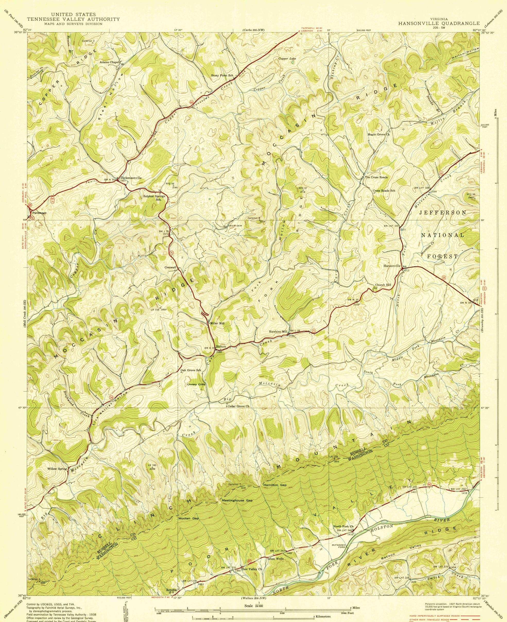
by stereophotogrammetric process. Field examination by Tennessee Valley Authority - 1938 Office inspection and review by the Geological Survey. Engraved and printed by the Coast and Geodetic Survey.
